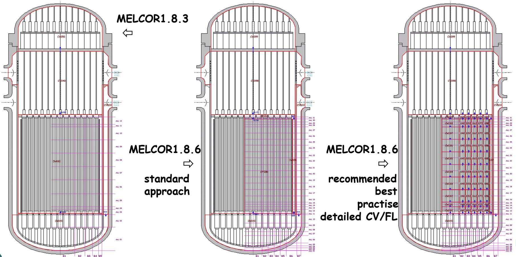
Reactor Pressure Vessel Nodalization - RPV Figure, COR, CVH/FL Packages
