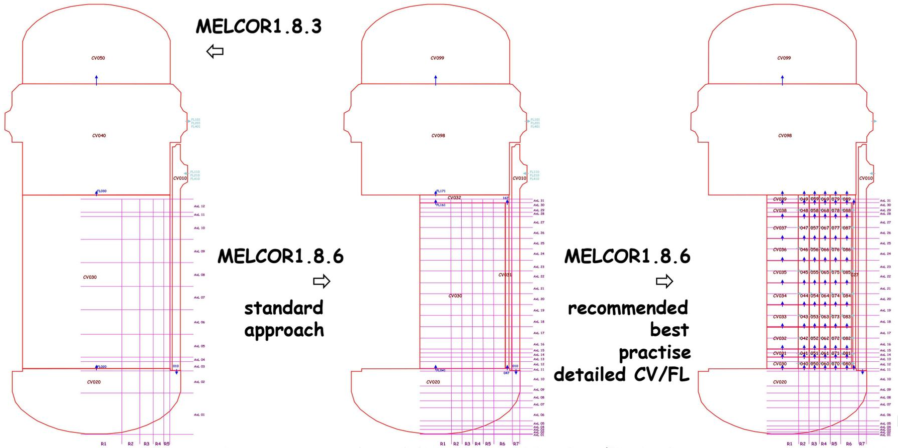
Reactor Pressure Vessel Nodalization - COR, CVH/FL Packages
