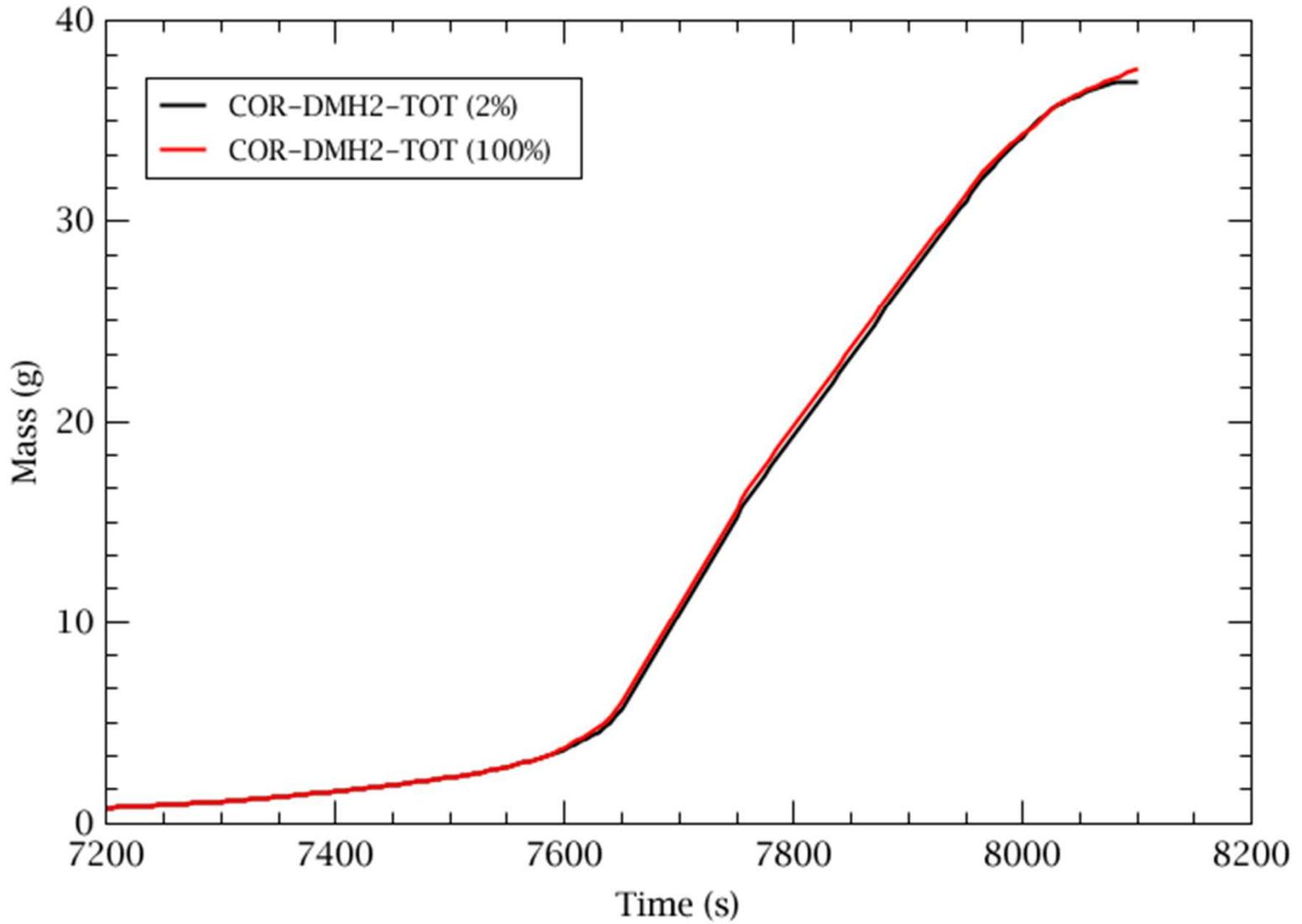
Threshold temperature for oxidation of boron carbide - effect on the mass of carbon gases and hydrogen
