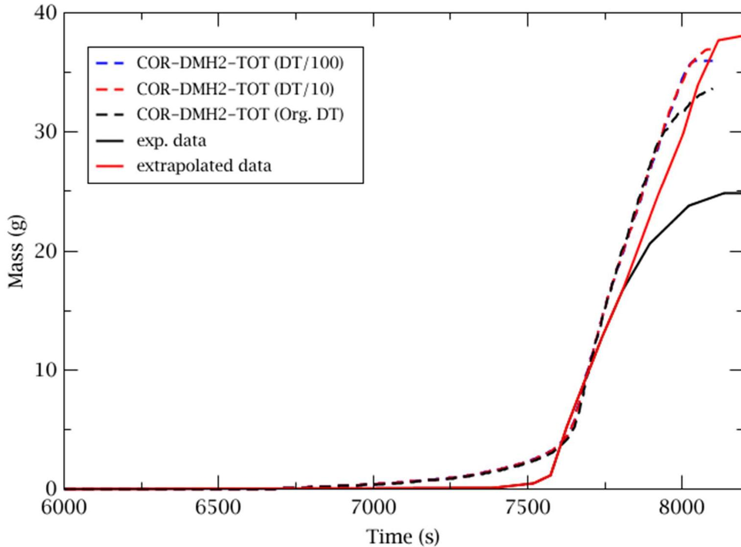
Available fraction of boron carbide for the oxidation with steam - effect on the mass of carbon gases and hydrogen
