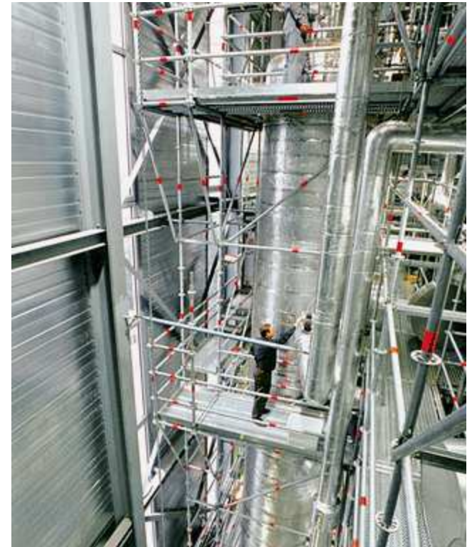
Large-scale facility PANDA: drawing off heat by natural circulation
