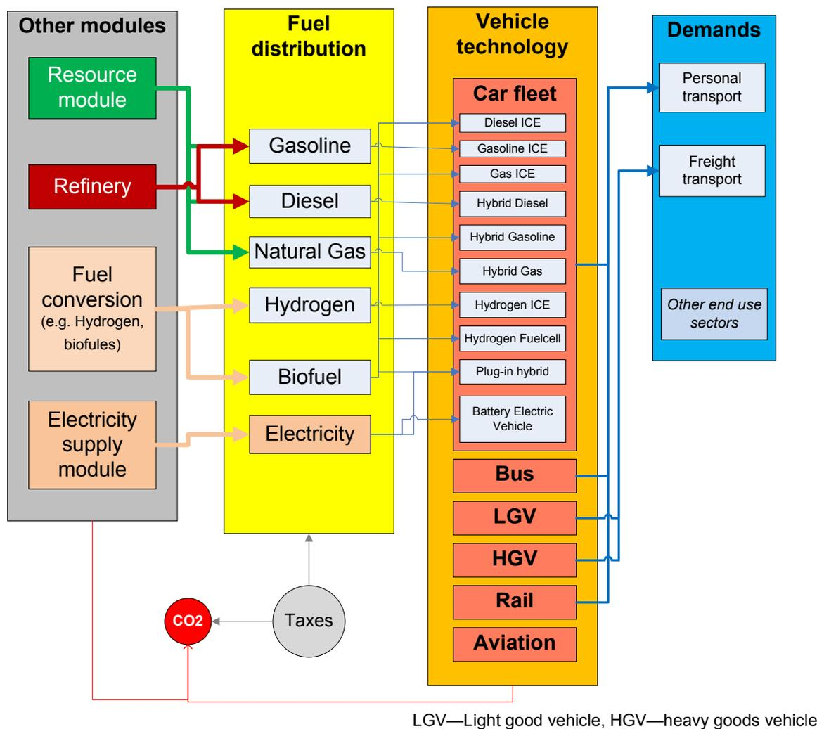
Figure 18: Simplified RES of the transport module
