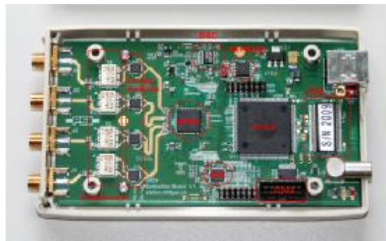
Figure 4: DRS4 evaluation board with four input channels and USB 2.0 readout
