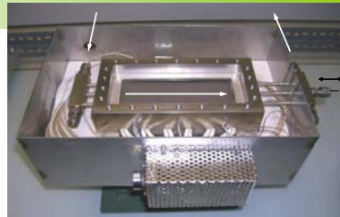
Channel reactor with catalytic plate (insulation removed). The white arrows visualize the flow through the reactor. On the right side of the reactor the septum port with the movable sampling capillary (black arrow) is visible
