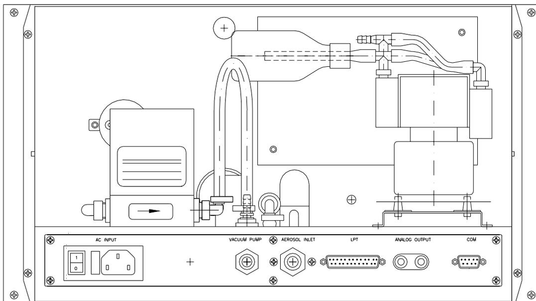
Figure 6 : Rear View – Interior – instrument configured for ‘External Pump’
