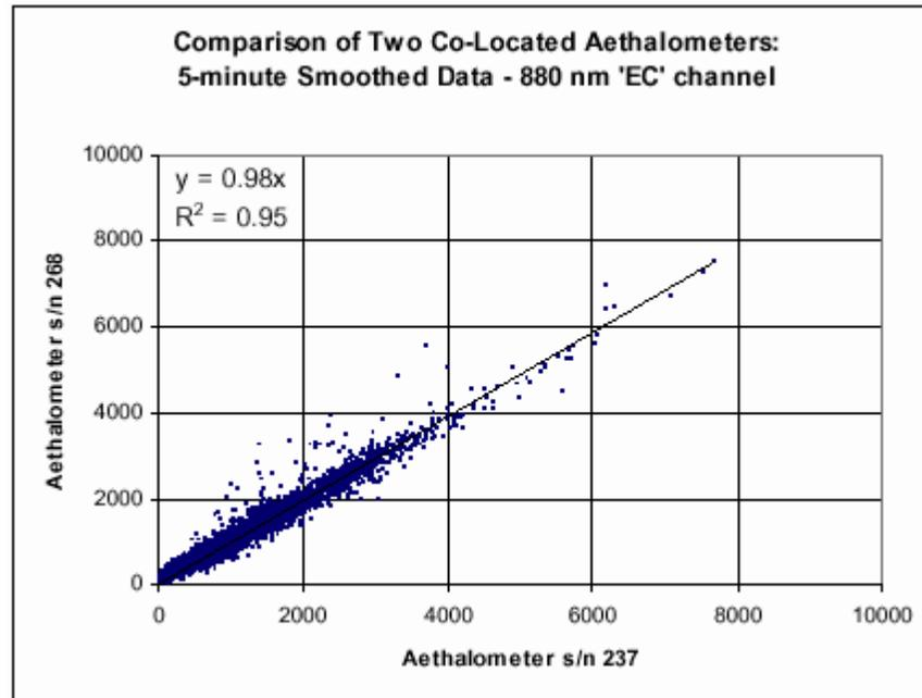
Comparison of data from two co-located Aethalometers under test at the ETV Pittsburgh site.
