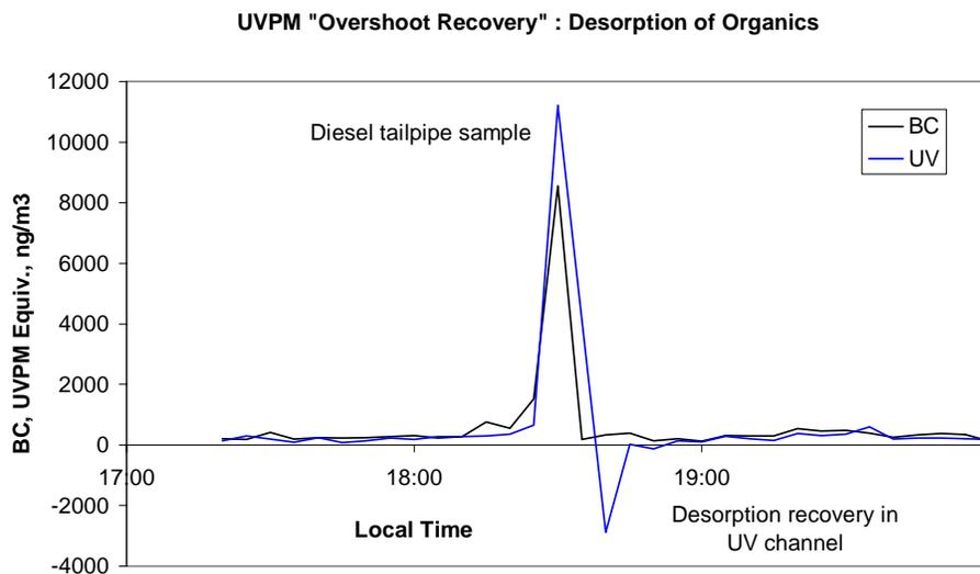
vicinity of a diesel engine tailpipe, the UV data showed a 'negative' recovery. This is not an instrumental error, but indicates that UV-absorbing material was deposited on the filter spot during the sampling event, and then desorbed from the filter spot afterwards.
