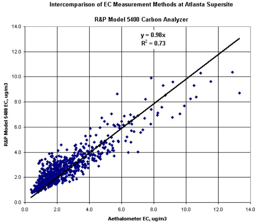
Intercomparison of Aethalometer data with ‘R&P 5400’ thermal EC analyzer
