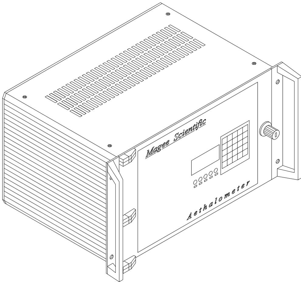
The Aethalometer™ - 19-inch rack mount chassis version
