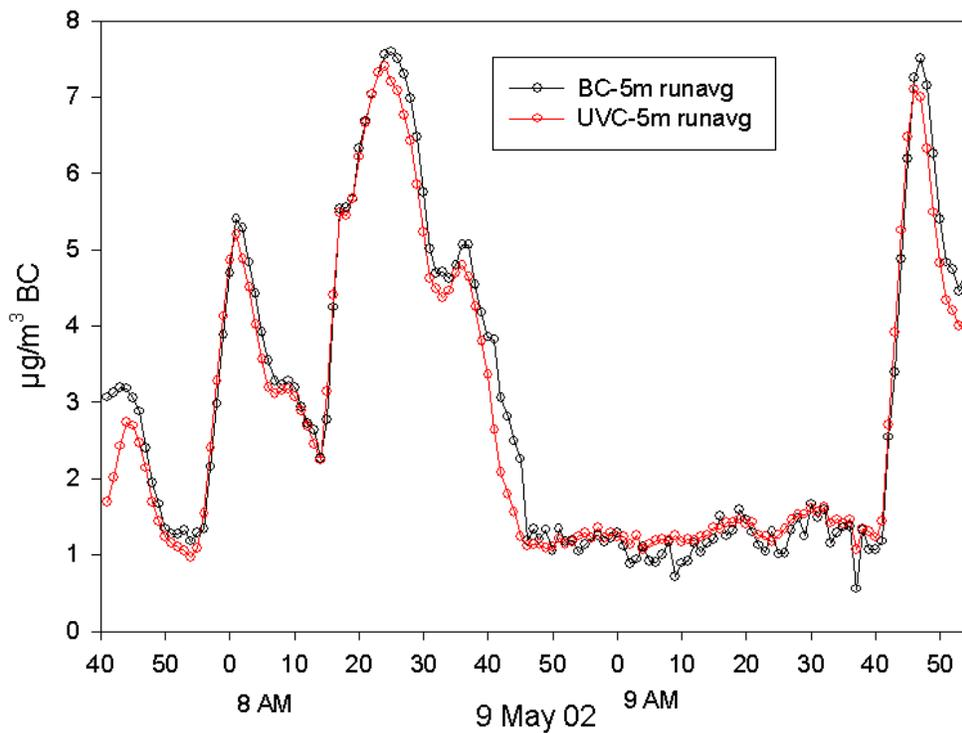
Measurements in car on highway during morning commute, Boston, MA, area.
