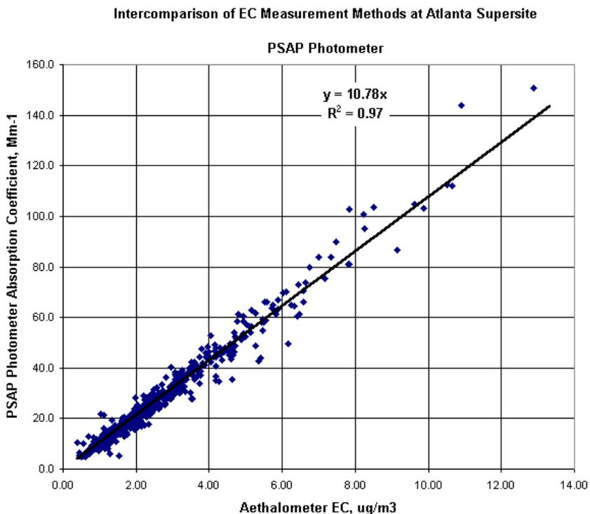
Intercomparison of Aethalometer data ( $\mu\text{g}/\text{m}^3$ )
