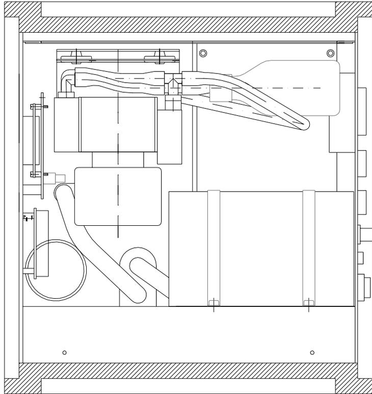
Figure 17 : 'Portable' Aethalometer™ - right side interior
