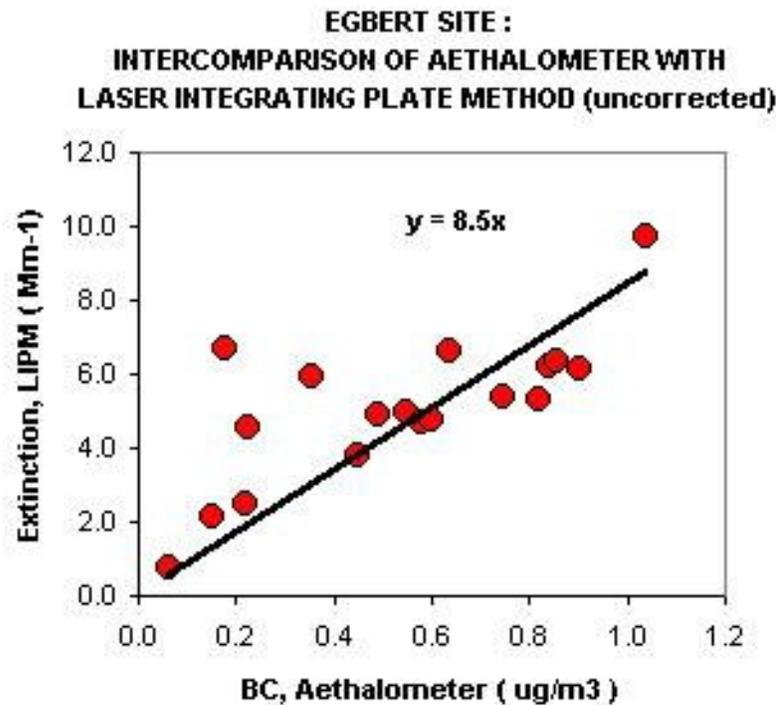
Intercomparison of Aethalometer data ( $\mu\text{g}/\text{m}^3$ )
