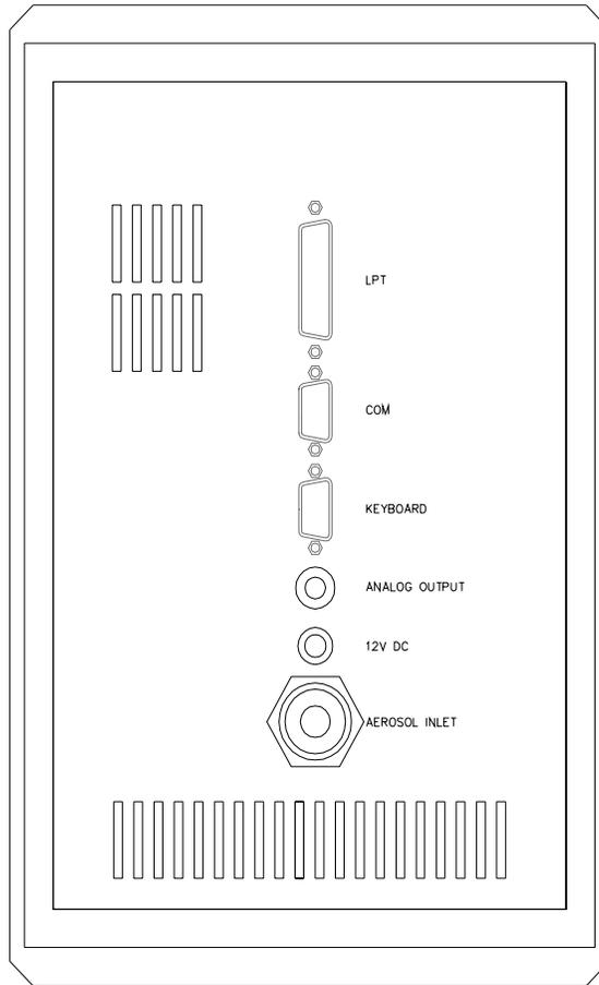
Figure 19 : 'Portable' Aethalometer™ - rear view
