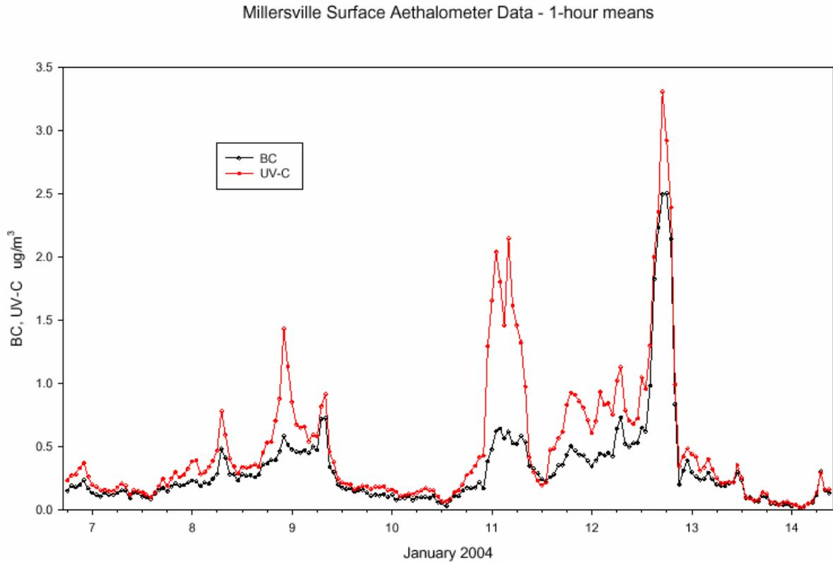
The final figure illustrates 'Spectrum' 7-wavelength Aethalometer data taken in an urban location where the aerosol is essentially uniformly absorbing across the wavelength range from 370 to 950 nm. The tracking of the data in all seven wavelengths vindicates the assumption of the  $1 / \lambda$  dependence of absorption.
