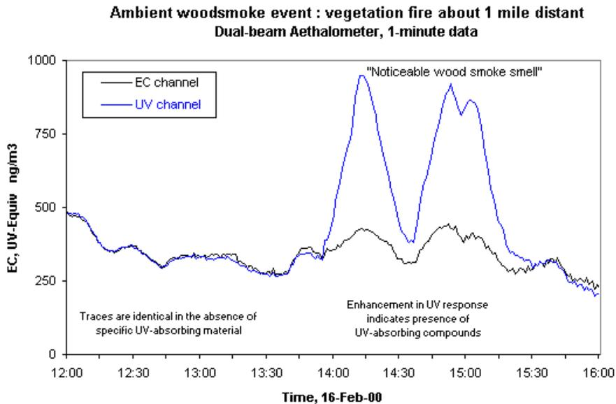
Dual-wavelength Aethalometer data during impact of smoke from burning vegetation.
