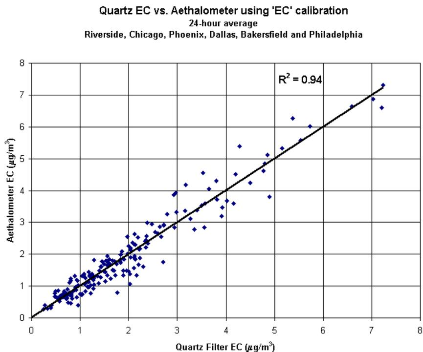
Intercomparison of Aethalometer data with ‘TOR’ analysis of parallel samples:
