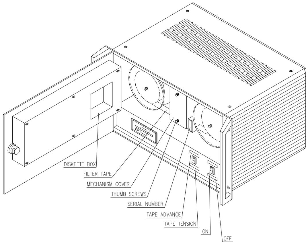
The Aethalometer™ - 19-inch rack mount chassis version
