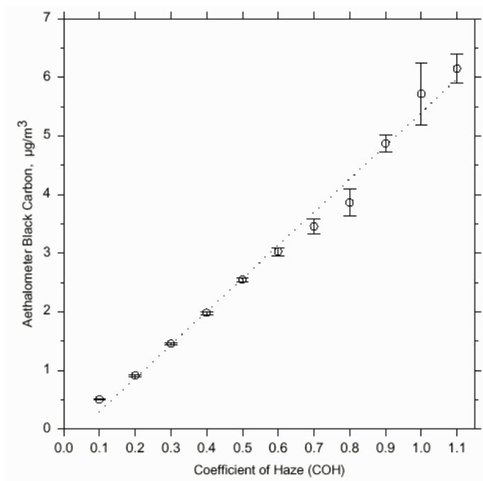
Intercomparison of Aethalometer ( $\mu\text{g}/\text{m}^3$ ) with Coefficient Of Haze tape sampler (COH): from Allen, Lawrence, and Koutrakis, "Field Validation...", *Atmos. Env.* **33**: 5 (Feb 1999).
