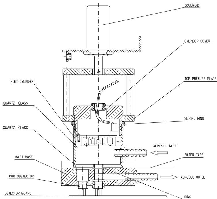
Figure 13 : Cross-Section of Optical Analysis Head (diagrammatic only)
