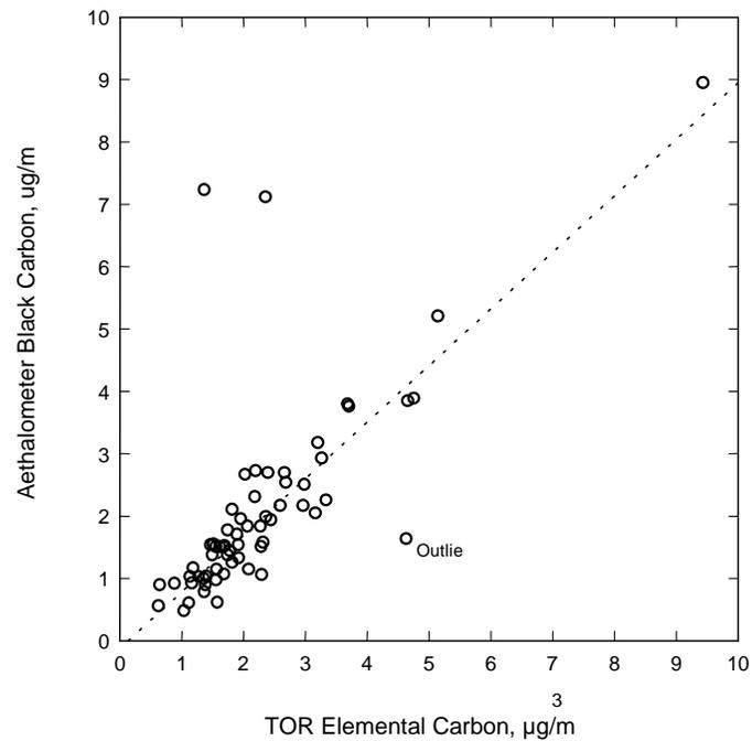
Intercomparison of Aethalometer data with 'TOR' analysis of parallel samples:
