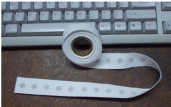
Filter tape spots: “High Sensitivity” 0.5 cm<sup>2</sup> spot size.
