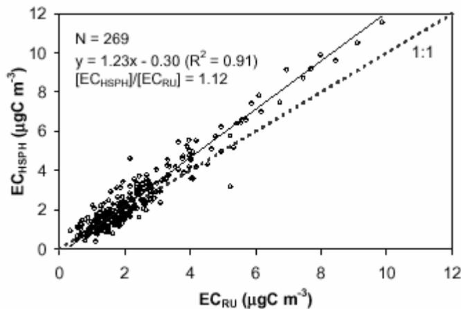
At the same ‘Atlanta Supersite’ intercomparison, a filtration-based thermal analyzer was operated by Rutgers University. Comparison of this data (‘RU’) with the Aethalometer (operated by Harvard, ‘HSPH’) also showed excellent agreement.
