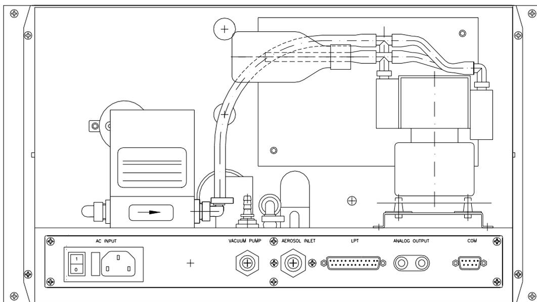
Figure 7 : Rear View – Interior – instrument provided with Internal Pump
