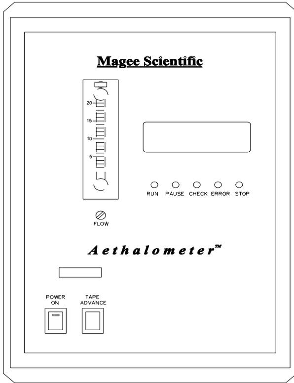
Figure 18 : 'Portable' Aethalometer™ -front view
