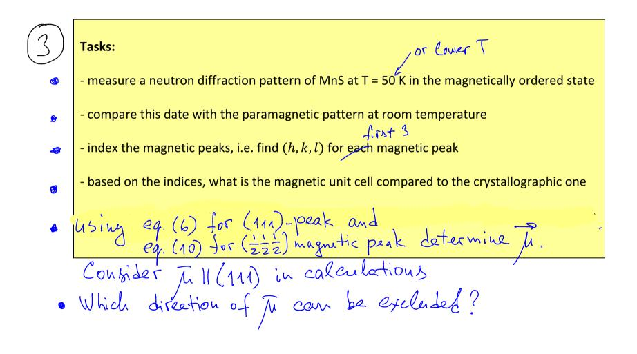
Task 3: Indexing of the magnetic Bragg peaks. Calculation of magnetic structure factors and determination of the value and direction of the Mn-spins.
