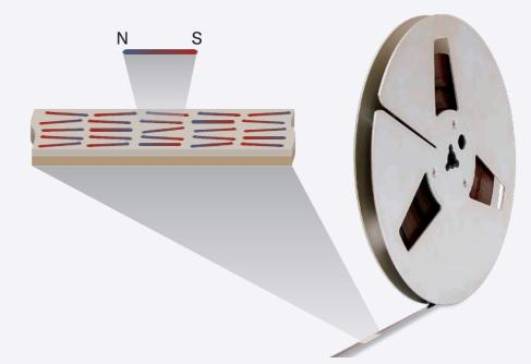
Magnetic tapes are made up of a layer of tiny magnetic particles – like little compass needles that can be oriented to store information. To make recordings on old and unreadable tapes audible again, Sebastian Gliga uses synchrotron light from the Swiss Light Source SLS.
