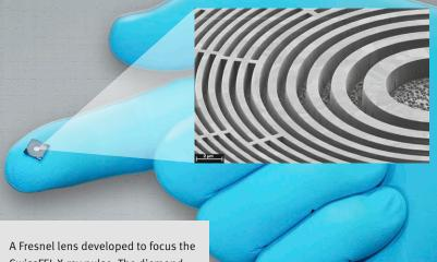
A Fresnel lens developed to focus the SwissFEL X-ray pulse. The diamond layer was structured using a lithographic process in order to make the focussing possible. 1 µm (micrometre) is equal to one thousandth of a millimetre.
