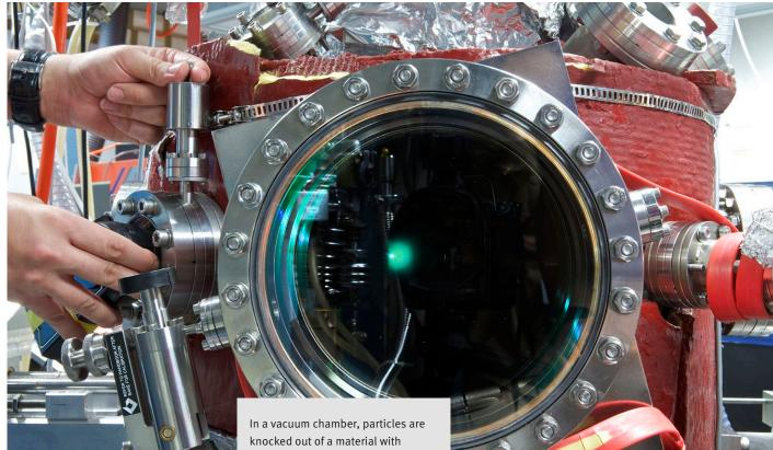
knocked out of a material with the help of a laser. The particles emit green light on their way from the material to the sample holder (from left to right).
