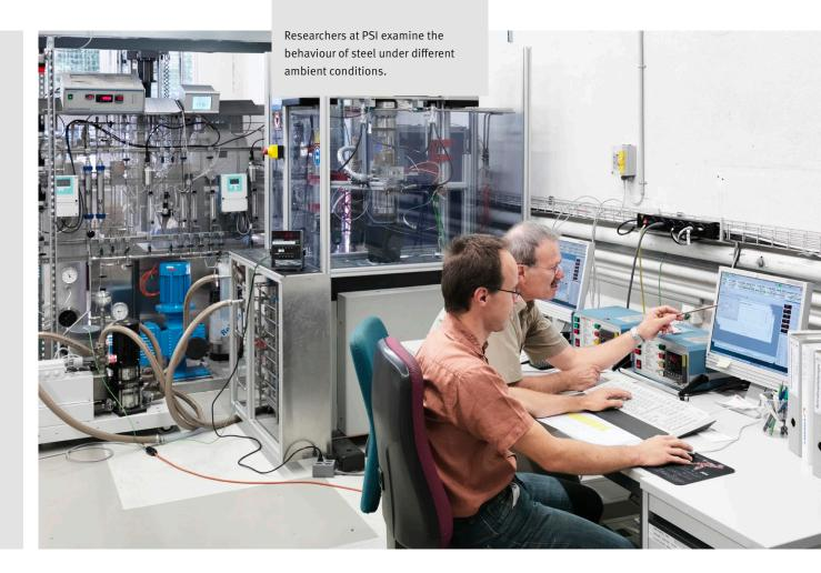
Steel is tested in this facility under conditions which occur in nuclear power stations. The results are incorporated in mathematical models with which the safety, and therefore the lifetime, of a nuclear power plant can be estimated.
