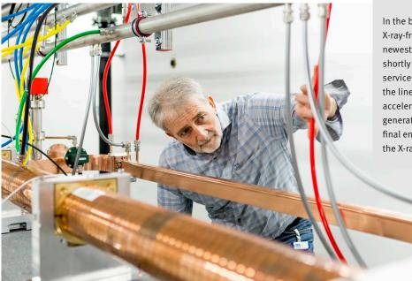
In the beam tunnel of the SwissFEL X-ray-free-electron laser, the newest large research facility of PSI, shortly before it was brought into service. Visible here is part of the linear accelerator. The linear accelerator brings the previously generated electrons up to the final energy required. Only then can the X-ray light be generated.
