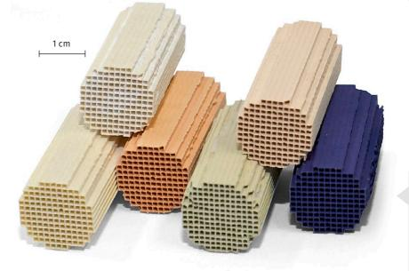
Different catalysts coated onto ceramic honeycomb bodies (far left: uncoated). The colour varies according to the chemical composition of the catalysts.
