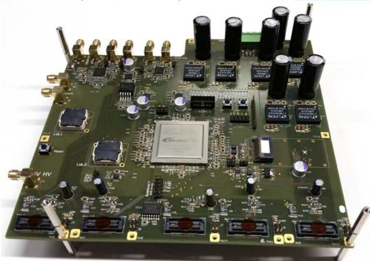
Prototype based on Altera/Intel Stratix IV FPGA
