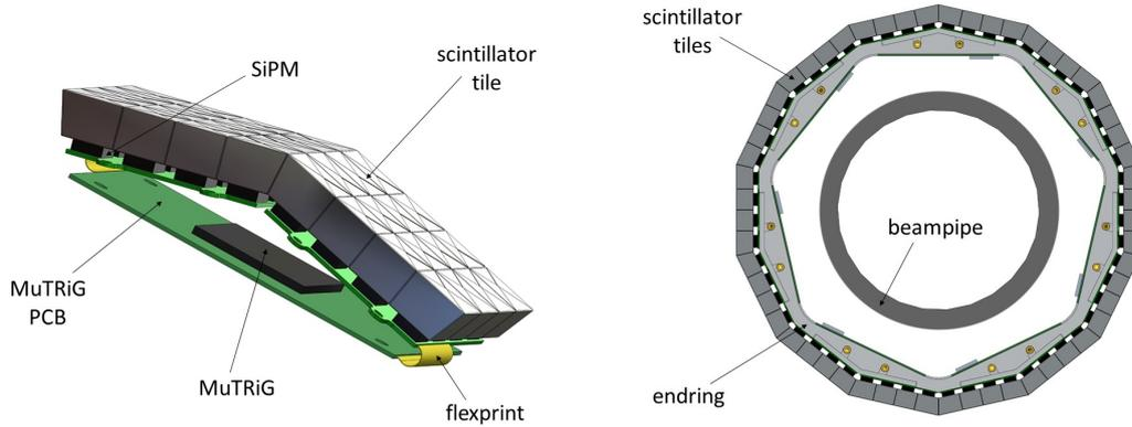
**Figure 2.9** – A submodule of the  $MU3E$  tiles detector. Seven such modules arrange in a ring around the beam pipe. The ring structure is replicated 14 times along the beam direction in both recur stations. Figure source [38]
