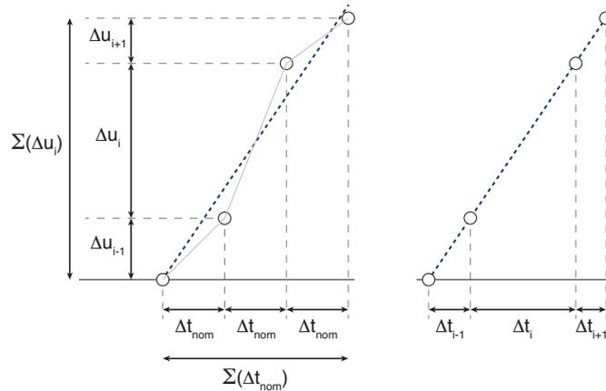
**Figure 5.8** – Illustration of the local time calibration algorithm [77]. Knowing the difference between voltage levels allows time intervals to be adjusted such that the points in the figure lie on a straight line. The shape of the line is known because the calibration happens only in the sections of the sine signal that can be approximated well by a straight line.
