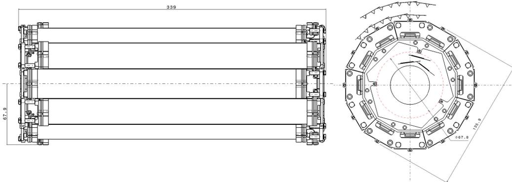
**Figure 8.2** – Dimensions of the SciFi detector. The length of 339 mm is fixed by the outer pixel support and the tiles detector. The hexagonal beam pipe and the third pixel layer determine the inner (33.9 mm) and outer (67.9 mm) radii of the detector components. Module elements from each of the outer and inner pixel layers are shown in the cross-section view for reference.
