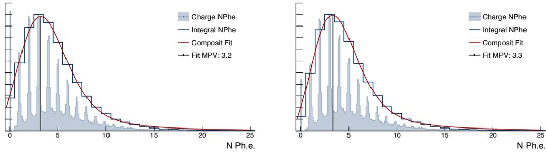
**Figure 6.10** – Photoelectron spectra of fiber with maximum charge per cluster for one side of a ribbon with a single fiber readout. Clustering algorithm assumes  $OR$  coincidence,  $Th^{all} = Th^{seed} = 0.5$  ph.e. and multiplicity  $\geq 1$  (Left) or multiplicity  $\geq 2$  (Right). The data is generated with  $Ribbon_{TiO_2}$  ribbon.
