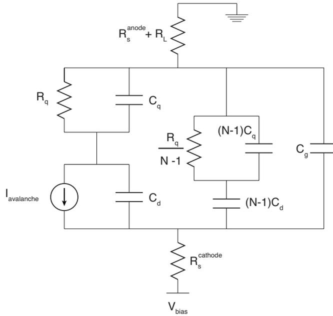
**Figure 4.12** – Equivalent circuit of an SiPM with large number of  $N$  parallel-connected Geiger mode APD [70]. The values provide by the vendor HAMAMATSU for the S1352 HQR are the following:  $N = 104$ ,  $C_d = 115$  fF,  $C_q = 18$  fF,  $C_g = 1$  pF,  $R = 470$  k $\Omega$ ,  $R_s^{\text{cathode}} = 0.5 \Omega$  and  $R_s^{\text{anode}} = 1.5 \Omega$ .
