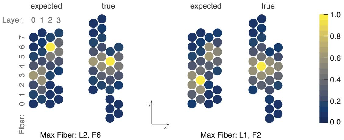
**Figure 6.3** – An example of a ribbon where the fibers that have been chosen for the fanout are not staggered as expected. By looking at the hit distribution intensity in neighboring fibers the true positions of the fanned out fibers are reconstructed. This cross-section is produced with the *RibbonClear* ribbon.
