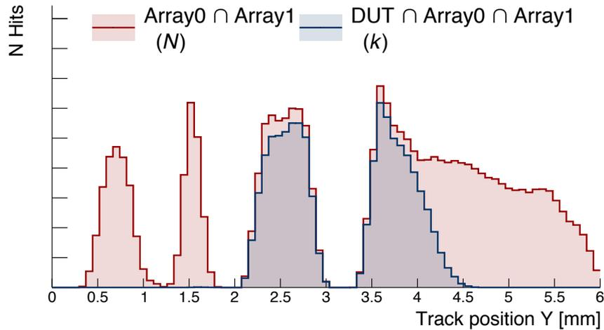
**Figure 6.6** – Number of tracks (—) defined using conservative cuts (see text) on the hits of *Array\_0* and *Array\_1*. Hits in the DUT matched with tracks (—) if the deviation from the track predicted position for the hit is within 0.5 mm. The empty regions correspond to locations with dead channels in either of the arrays.
