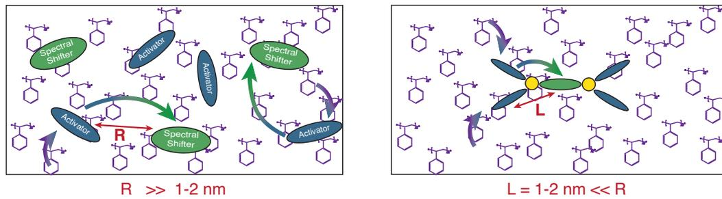
**Figure 3.3** – Schematic representation of a plastic scintillator based on polystyrene with traditional activator and spectral shifter luminophores (Left). The novel NOL molecules combine both the activator and the shifter in a single nanostructure increasing the efficiency of the wavelength shifting process. Figure adapted from [55]
