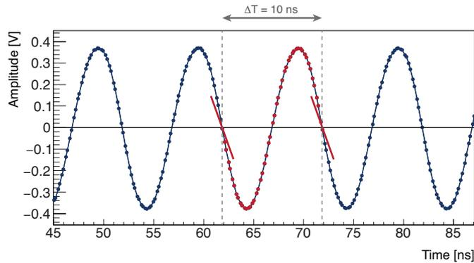
**Figure 5.9** – Illustration of the global time calibration algorithm [77]. The period of the sine is fixed. Any deviation of the measured period from the expected one is factored as a small correction to all time intervals between the start and end of a period.
