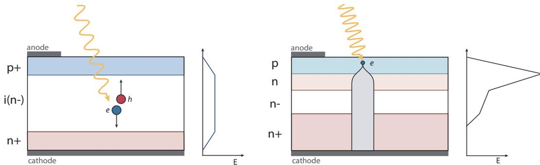
**Figure 4.2** – Schematic of the electric field and doping of a PIN diode (Left) and an APD (Right). In the former the electrons and holes drift towards the cathode and anode without multiplication. In the later an avalanche proportional to the incident light flux is triggered by the electrons under the high intensity electric field at the PN junction.
