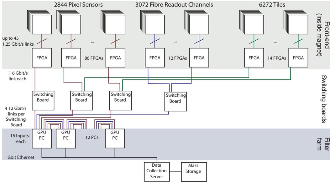
Figure 2.11 – Overall readout scheme of the Mu3E detectors.
