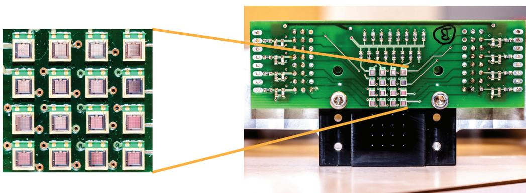
**Figure 4.7** – A photo of a  $4 \times 4$  matrix assembled with 16 S12571-050P MPPCs. All sensors are biased via a common voltage source while the signals are individually transmitted to an amplifier.
