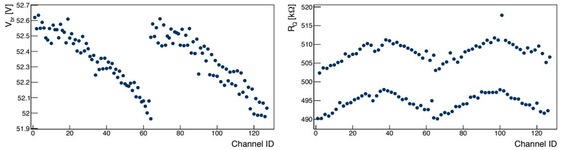
Figure 4.10 – Breakdown voltage (Left) and quenching resistor (Right) values measured for all 128 channels of a Hamamatsu S13552-HRQ. The repetitive pattern is due to the two dies constituting a single device.
