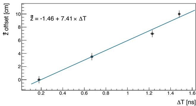
**Figure 7.21** – Time difference offset caused by particles traversing the ribbon at different offsets along  $\bar{z}$ . The zero position is the middle of the ribbon. Results are acquired using a three layer SciFi ribbon made of SCSE-78MJ fibers.
