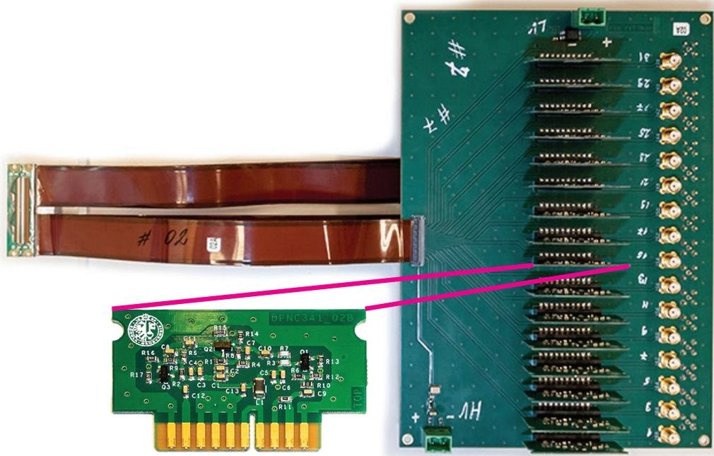
**Figure 4.13** – A photo of the modular amplifier PCB developed for the array SiPMs. The board houses 32 plug-gable amplifiers, 16 on each side. A HAMAMATSU S13552 array soldered on a custom PCB with four flex prints, each carrying 32 signal lines, is also connected to the amplifier board.
