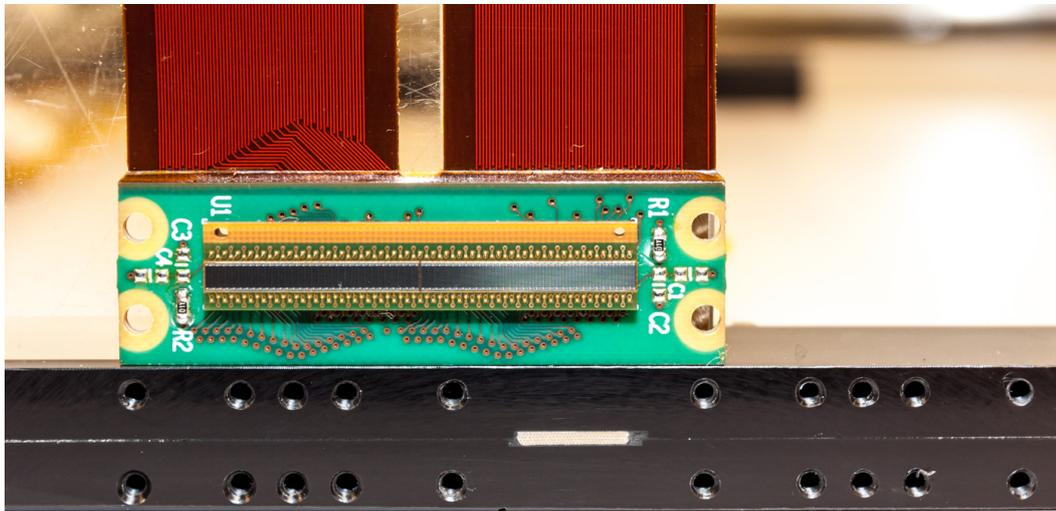
Figure 4.11 – Assembly between SiPM arrays mounted on custom PCBs and the fiber ribbon prototypes built and characterized within the current work.
