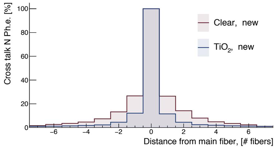
**Figure 6.12** – Percentage of light registered through fibers in one layer. The central bin corresponds to the main fiber in every event where the highest number of photoelectrons is recorded. Adding 20 %  $\text{TiO}_2$  powder to the epoxy while gluing the fibers into a ribbon reduces the crosstalk. The data is obtained from the two ribbons with *new* fibers.
