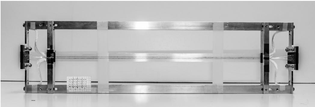
**Figure 3.10** – A full ribbon with single fiber readout.
