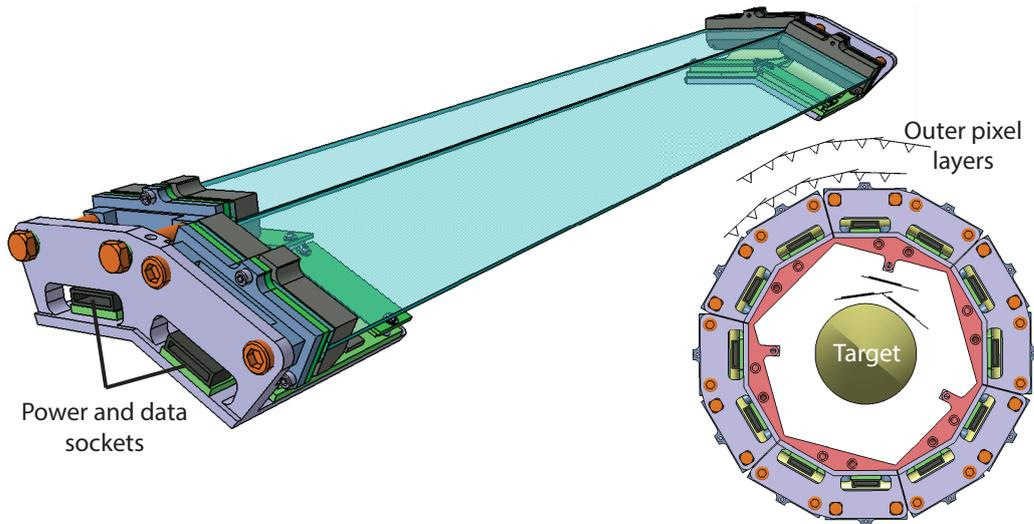
**Figure 8.4** – A SciFi detector module holding two ribbons staggered longitudinally to accommodate the SiPMs mounts. Six such modules arrange on top of the SciFi support/cooling ring.
