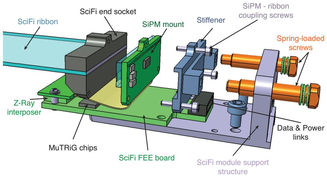
**Figure 8.6** – An exploded view showing the end piece assembly of one ribbon in a fiber module. The coupling between the SiPM and the polished ribbon surface is static, while the large spring loaded screws prevent sagging of the fiber mat under thermal expansion. The SciFi ribbon is installed on one side of the L-shape module support.
