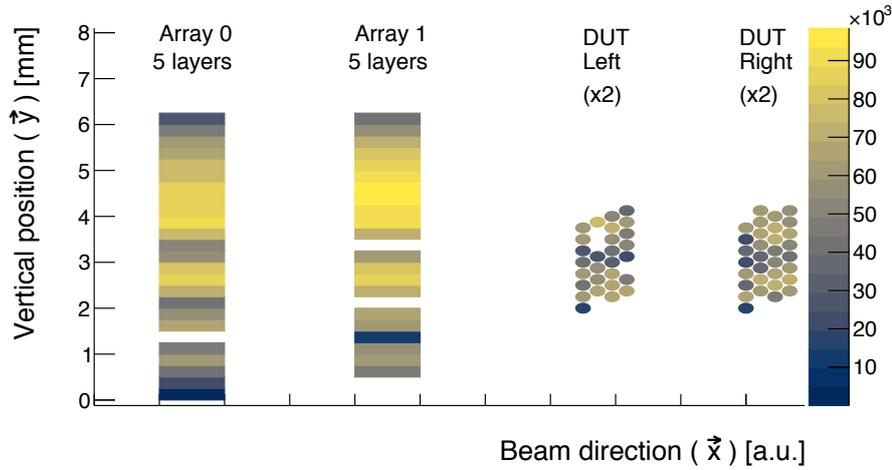
**Figure 6.5** – Number of hits recorded in each detector channel during one run. The arrays exhibit higher number of hits per channel due to the larger effective area of the photosensor which couples to several fibers per channel while in the single fiber readout individual fibers are matched to separate SiPM channel. The DUT is *Ribbon<sub>TiO<sub>2</sub></sub>* ribbon and the S12571-050P photosensor are reverse biased at  $V_{br} + 2$  V.
