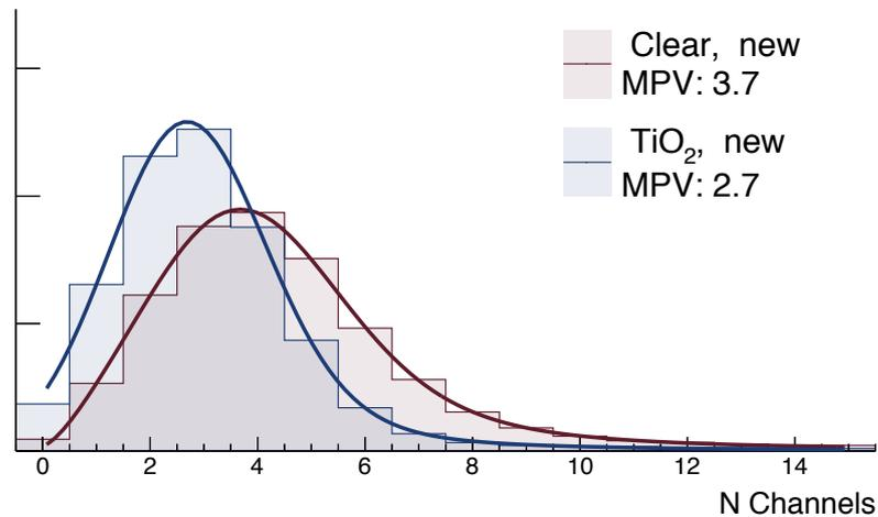
**Figure 6.13** – Event multiplicity as seen on one side of the ribbons with *new* fibers. The photoelectron threshold is 0.5 ph.e. Entries in the zero bin are added only if a cluster is found on the opposite side but not in the currently analyzed one. The data is modeled with a convolution of a Gaussian and Landau distributions with the MPV of the fit reported in comparisons between samples.
