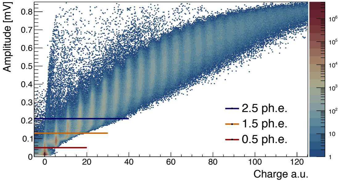
**Figure 7.6** – Charge vs maximum amplitude for all 32 SiPM channels attached to one side of a SciFi ribbon. The current sample present events collected when the active area of the SciFi ribbon has been traversed by beam particles. The thresholds corresponding to 0.5 ph.e. (—), 1.5 ph.e. (—) and 2.5 ph.e. (—) have also been marked.
