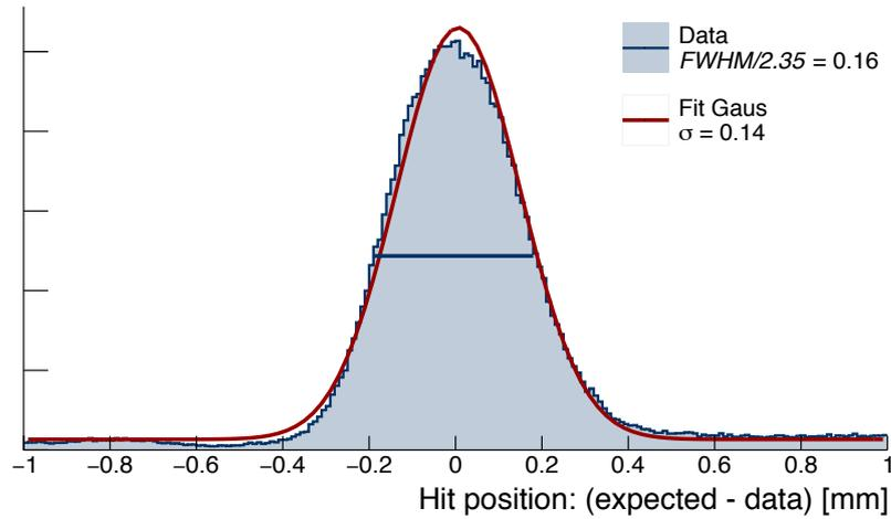
**Figure 6.7** – Deviation between the predicted position of a hit in the DUT and the actually observed one. Only hits with residuals in the range (-0.5 mm, 0.5 mm) are used in the subsequent efficiency studies.
