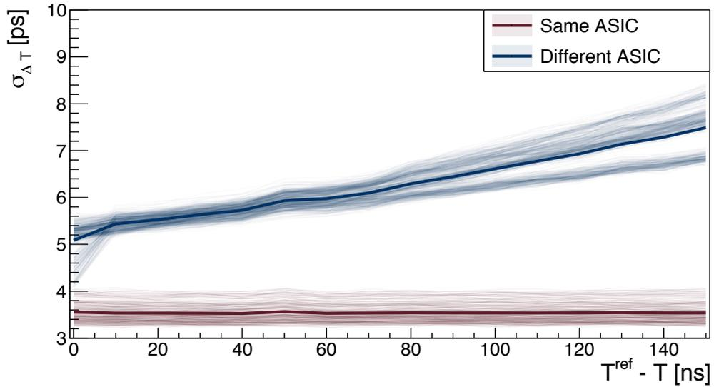
**Figure 5.13** – Time difference jitter scan as a function of the distance to the reference signal and the measured one. The jitter is expressed as the value of the standard deviation in Gaussian fitted time difference histograms. Depending on the relative time displacement between the reference signal and the test signal a small increase in the jitter is observed.
