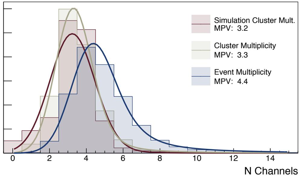
**Figure 7.14** – The cluster multiplicity obtained during the test beam at PSI (—) is reproduced through simulation (—) with the main Mu3E simulation framework. The event multiplicity (—) tends to be larger by approximately 30 %. The figure is adapted from [51] with test beam data provided by measurements performed in this work. A ribbon of four layers SCSF-78MJ is used in both studies.
