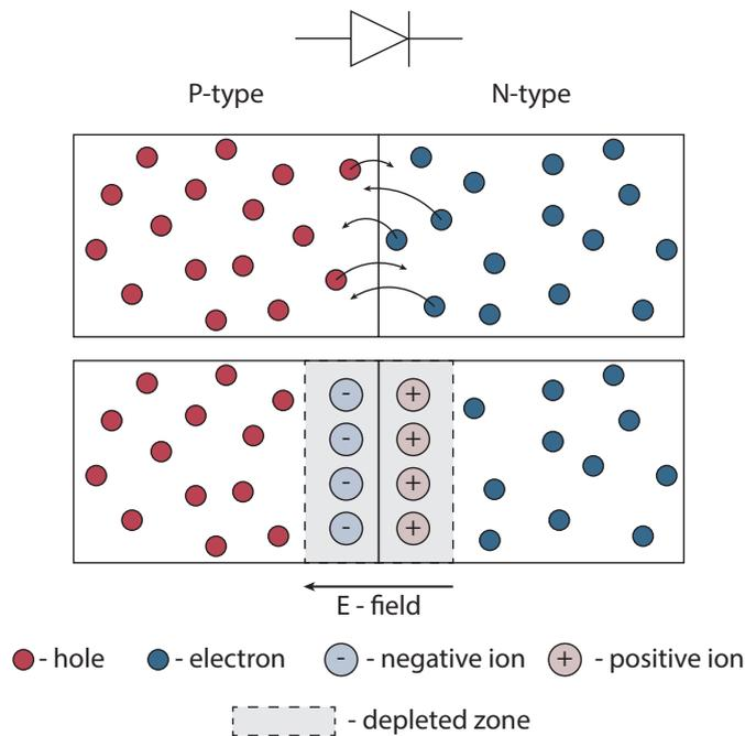
**Figure 4.1** – The excess of free electrons in the  $n$ -type semiconductor and holes in the  $p$ -type cause drift of the respective carries to the section with lower concentration. As a result, negative and positive ions are formed where holes ( $h$ ) and electrons ( $e$ ) have been replaced in the crystal lattice by the opposite carrier. The net effect is a volume depleted of free charges and a build-up of an electric field around the junction due to the newly formed ions.
