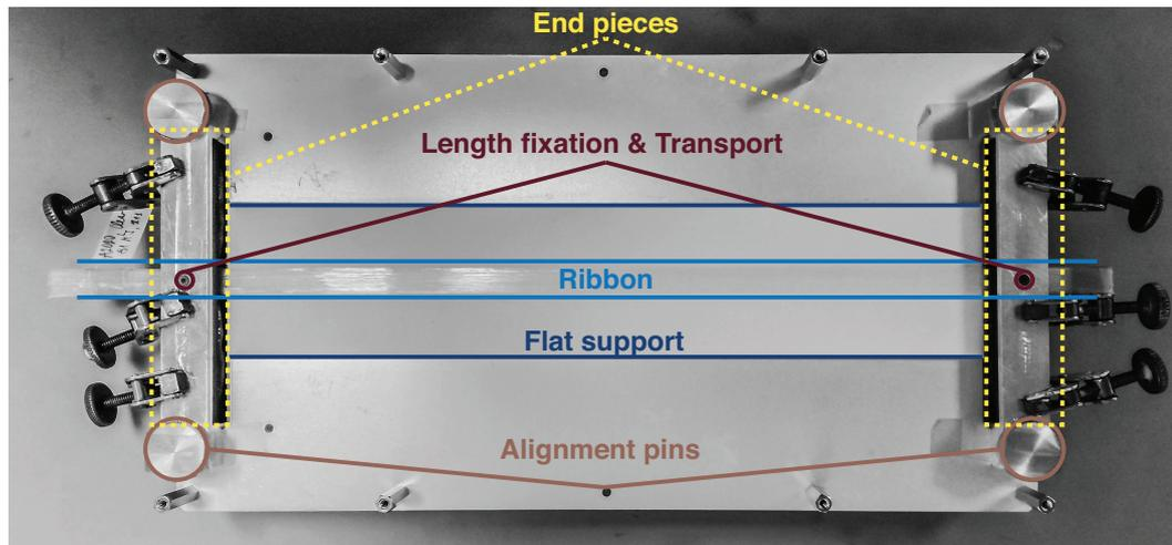
**Figure 3.11** – A jig used to position the end pieces on a ribbon with *column readout*. A length fixation is attached on top of the ribbon via the threaded holes in the end connectors. The ribbon lays flattened on a teflon plate while the epoxy in the connectors hardens.
