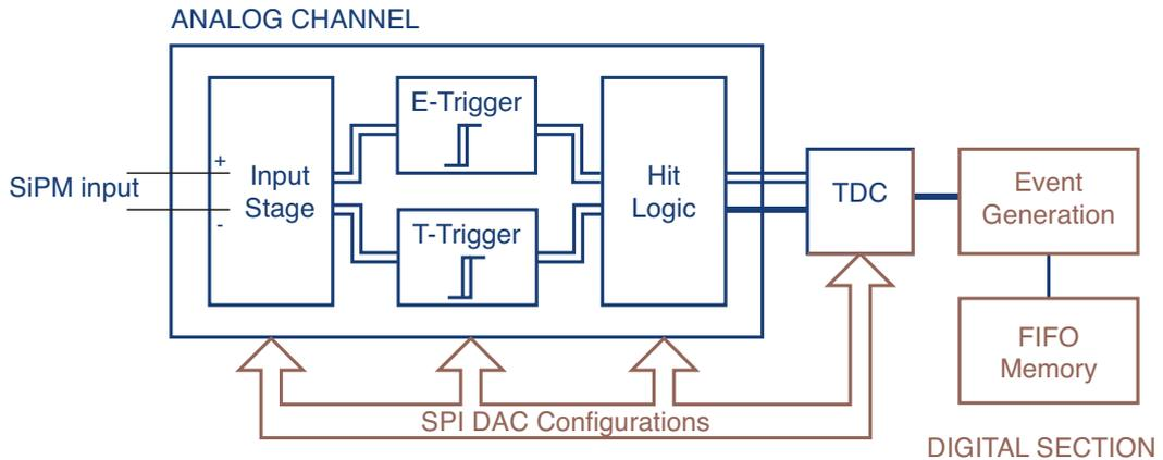
**Figure 5.14** – Block diagram of a single MuTRiG channel. Figure adapted from [43].
