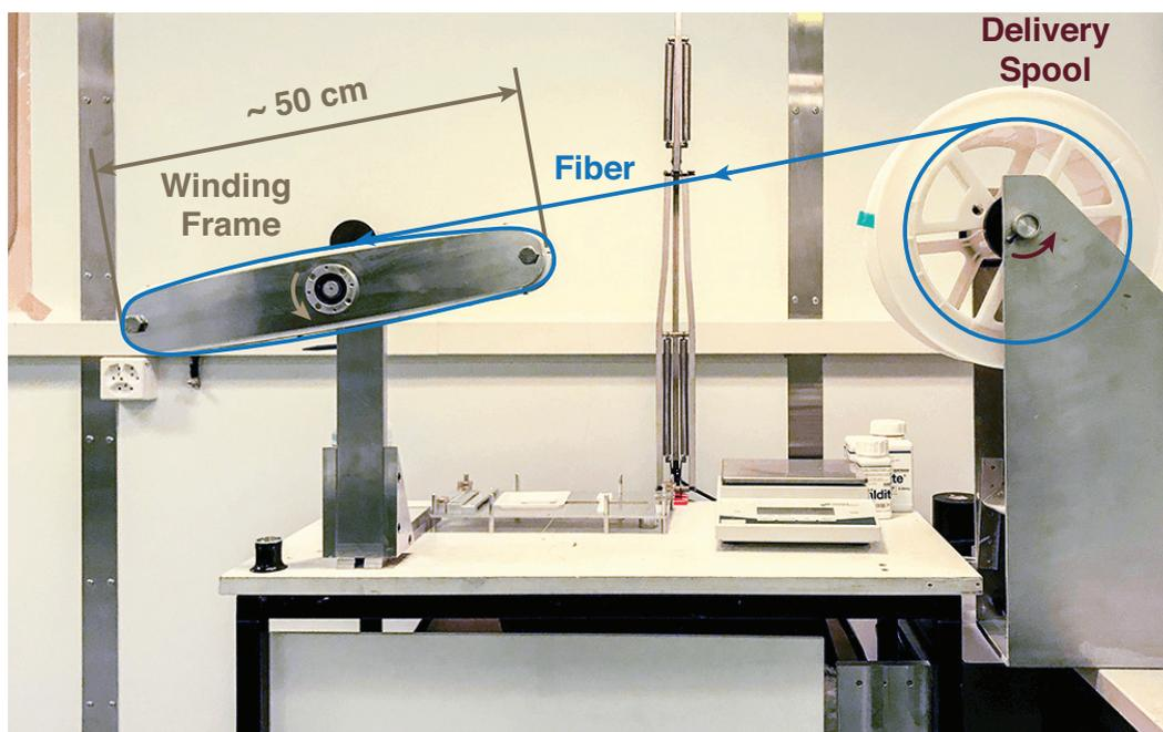
**Figure 3.6** – Fibers are drawn from the delivery spool (Right) and aligned next to each other in a U-shaped channel (Left) machined in a specially designed frame. Ribbons are assembled by winding one layer at a time.
