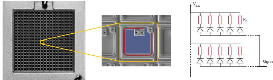
**Figure 4.4** – Each cell of a single channel SiPM device can be simplified as a diode in series with a quenching resistor. A matrix of cells connected in parallel constitutes a single channel SiPM. A practical realization of the quenching resistor  $R_Q$  (—) is marked on the microscopic image of a single G-APD cell. The shaded zone (—) marks the photosensitive area of the cell. Figure adapted from [62].
