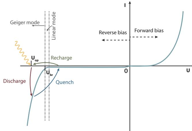
**Figure 4.3** – Biasing scheme of APD cells with an accent on the processes undergoing during Geiger mode operation. When a cell is biased above the breakdown voltage, a photon interacting in the active volume triggers a Geiger discharge which is subsequently quenched via a resistor. As a result, the electric field over the PN junction drops and a short recovery time is necessary before new avalanches can be formed.
