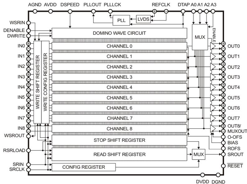
**Figure 5.3** – A functional diagram of the DRS4 ASIC [73]. The write signal for the sampling cells is generated by a chain of inverters on the chip and stabilized by a PLL. The content of the sampling cells can be send either to a multiplexed or individual output lines from where it is digitized with an external ADC.
