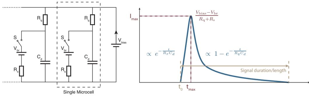
**Figure 4.6** – A simplified circuit of a G-APD microcell (Left) and a sketch of its output signal (Right). If several cells in an SiPM are triggered simultaneously, the output is a linear sum of all microcell responses.
