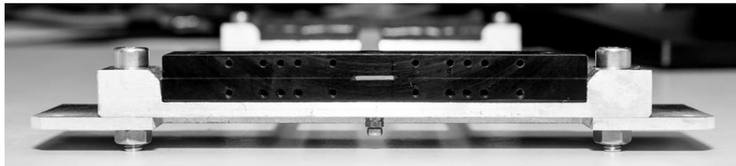
**Figure 3.12** – End piece socket mounted on a ribbon with column readout. The fixation screw in the bottom attaches the black connector to the alignment aluminum bracket. The holes on the front are used for coupling with the optical photosensor.
