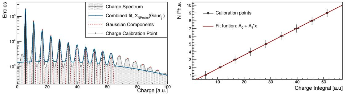
**Figure 7.7** – (Left) The charge projection of 7.6. Each peak is fitted with a Gaussian function and the centroid of the result is used as an input for the photoelectron calibration. (Right) The integrated SiPM signal shows expected linear proportionality to the generated number of photoelectrons.
