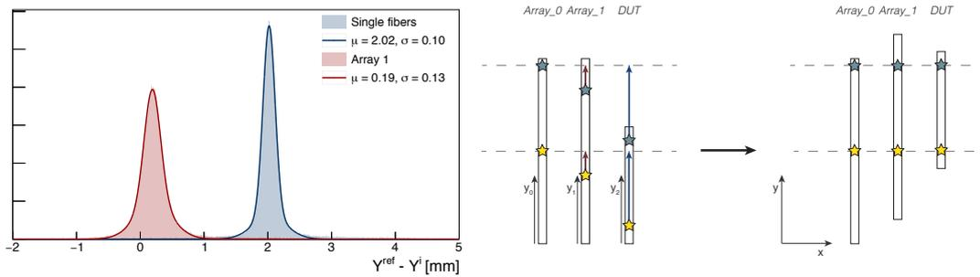
**Figure 6.4** – The plane of *Array\_0* is chosen as a reference and the alignment of the remaining two - *Array\_1* and the DUT - is reconstructed in software using the deviations between hit positions in each plane with respect to the reference.
