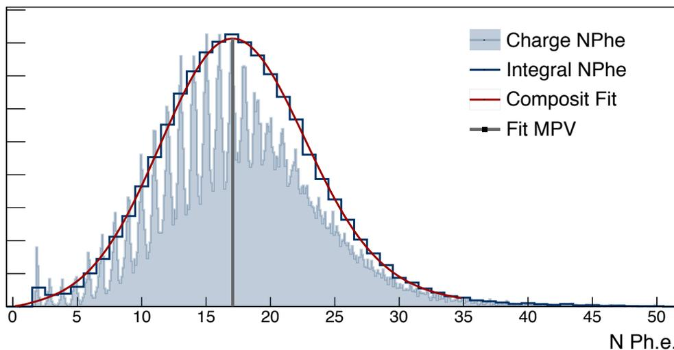
**Figure 7.13** – Cluster light yield of a three layered SCSF-78MJ fiber ribbon prepared with clear epoxy. The integral (—) NPhe is obtained by summing the charge in a region of  $\pm 0.5$  ph.e. around each integer. A convolution of a Gaussian and a Landau is used to fit the data (—) and the most probable value (MPV) is marked with a line —.
