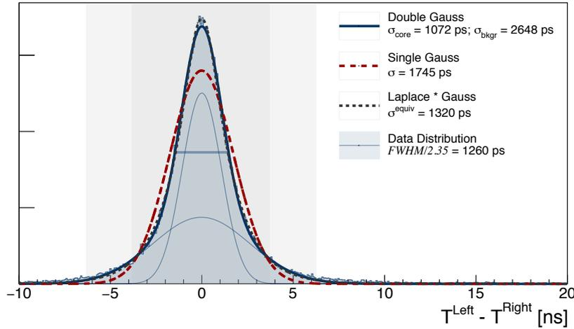
**Figure 6.11** – Time difference distribution using the **TFirst** algorithm on the *Ribbon<sub>TiO<sub>2</sub></sub>* ribbon. The data is best modeled with a convolution of a Laplacian and Gaussian, however, a double Gaussian (sum of two Gaussian distributions) is also an acceptable function and offers an intuitive interpretation of the fit parameters.
