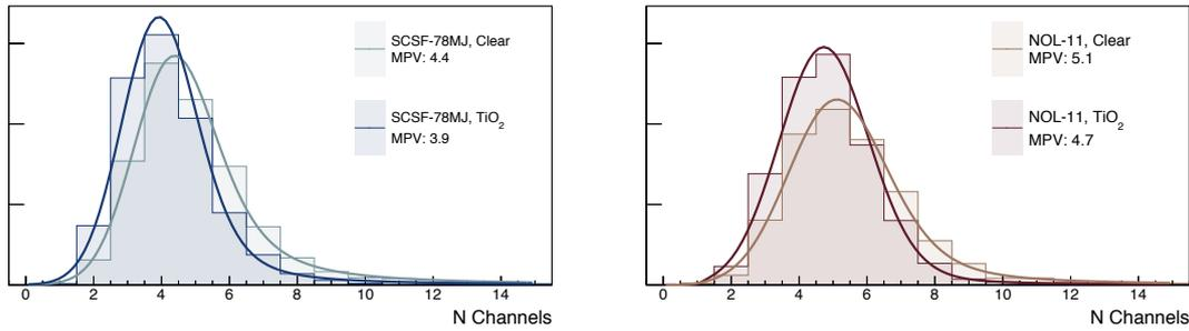
**Figure 7.15** – Event multiplicity at one side of a ribbon with four layers of SCSF-78MJ (Left) and four layers of NOL-11 (Right). Adding a TiO<sub>2</sub> powder in the epoxy with 20 % concentration by mass leads to reduction of the occupancy by  $\mathcal{O}(10\%)$  for 4 layer SciFi ribbon. The data is for particles traversing the ribbons at an angle of  $0^\circ$  and cluster threshold set at 0.5 phe.
