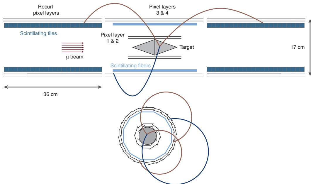
**Figure 2.3** – Schematic of the Phase I MU3E experiment.
