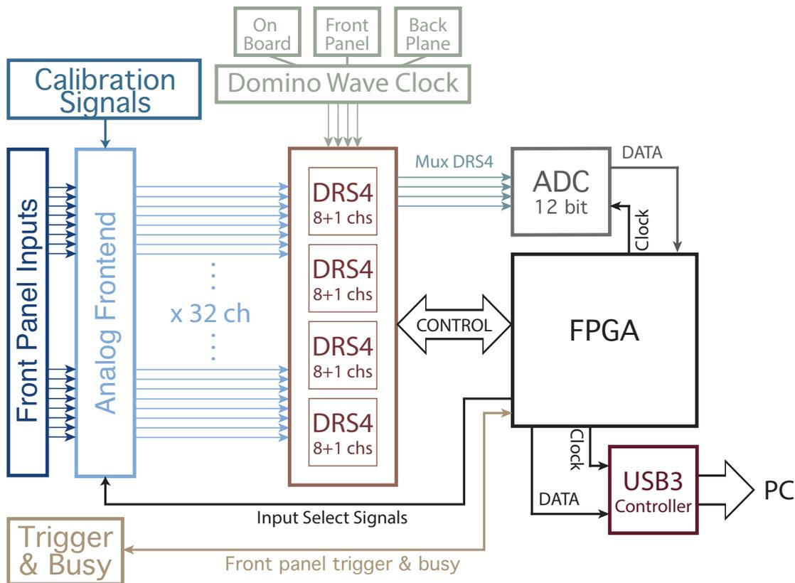
Figure 5.5 – Simplified schematics of the DPNC 342 readout board.
