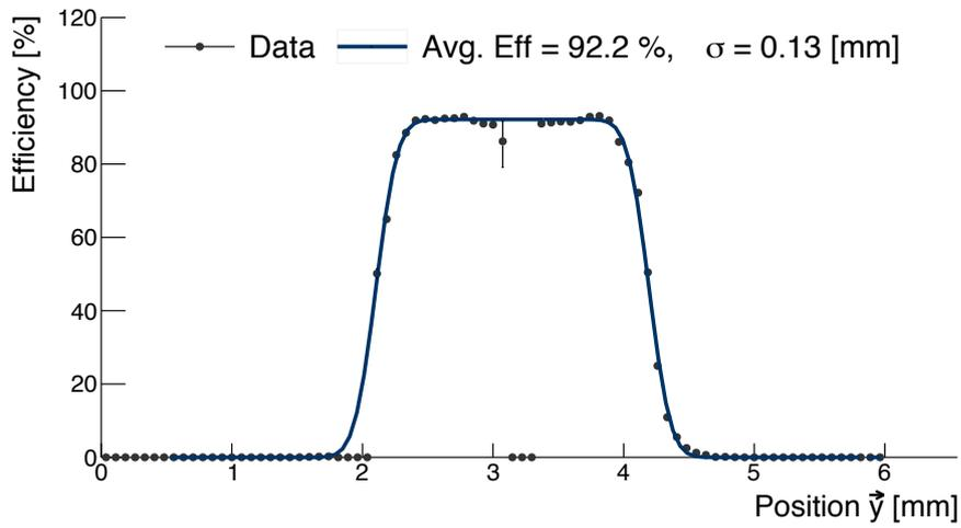
**Figure 6.8** – Sample efficiency profile scan along  $\vec{y}$  for  $New\_TiO_2$  ribbon. The data is modeled as a convolution between a square impulse and a Gaussian. The reported value of  $\sigma = 0.13$  mm is consistent with the position resolution of the tracker observed in previous plots.
