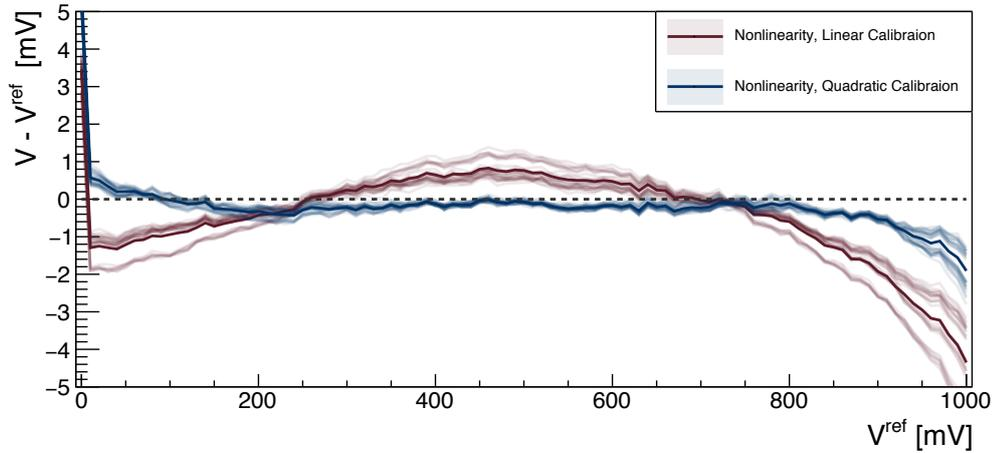
**Figure 5.6** – Nonlinearity of the voltage calibration depending on the model used for mapping the voltage value to the recorded ADC outputs. Using a quadratic function lead to better matching to a reference input signal. The data is from 64 channels in 8 DRS4 chips. A constant level reference signal is used for each point.
