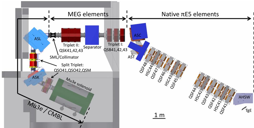
**Figure 2.5** – A CAD model of the full  $\pi$ E5 channel and CMBL. Positive muons produced in the TgE target (bottom right) are transported via existing  $\pi$ E5 elements, the beam line section shared with the MEG II experiment, and the dedicated CMBL to the MU3E solenoid. Figure source [40]
