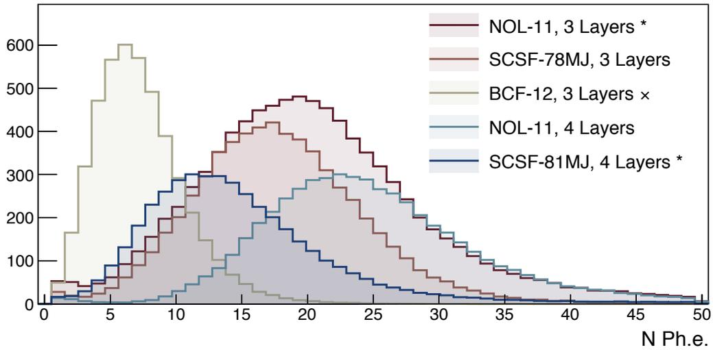
**Figure 7.17** – Light yield at one side of select ribbons. The number of photoelectrons is the charge sum of all channels in a cluster at one side matched to a track. The minimal cluster multiplicity is of two neighboring channels with an amplitude of at least 0.5 ph.e. The histograms are normalized by their integral. (\*) - ribbons with 20 % TiO<sub>2</sub> added to the glue. (x - individual fibers coated with  $\mathcal{O}$ (100 nm) of Al.
