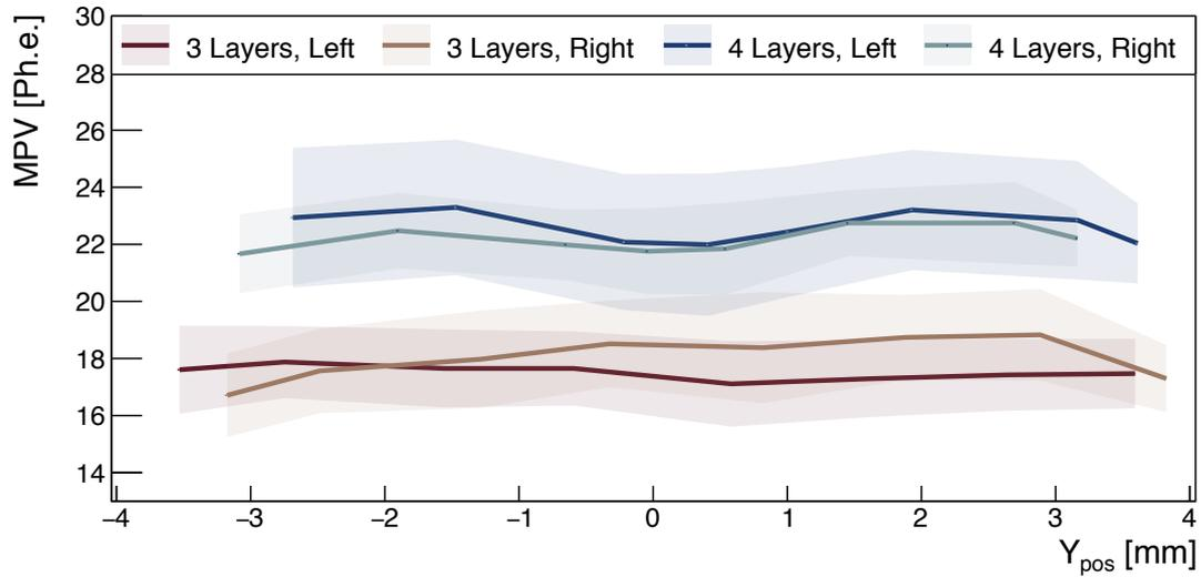
**Figure 7.20** – Cluster light yield for different ribbon positions scanned along the width of a SciFi ribbon. The left and right sides of two ribbons are plotted. One is composed of three and the other of four layers NOL-11 fiber, both prepared with 20 %  $\text{TiO}_2$  in the epoxy mixture.
