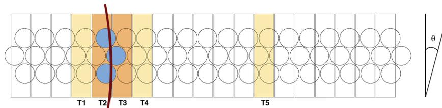
**Figure 7.10** – Transverse view of a three layered ribbon mapped to a SiPM array. A particle (—) traversing the ribbon generates scintillating light in some fibers (—) which can trigger signals in several SiPM channels (—, —). A "dark" count signal which is identical to a real event signal (—) should be excluded from the main cluster. Channels are first grouped by proximity and afterwards sorted by their timestamp.
