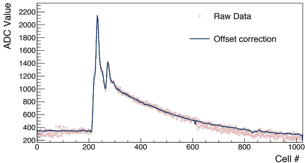
**Figure 5.7** – Comparison of a recorded waveform with and without voltage calibration. The shown calibrated data corrects only the offsets in each cells. However, the common baseline shift is not subtracted in order to illustrate the span of a single waveform in the ADC values. The scaling of the amplitude to voltage is omitted since it does not affect visible the shape of the shown result. The amplitude of the signal is about 500 mV.
