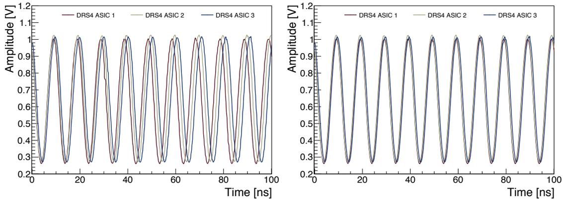
**Figure 5.10** – An identical sine signal distributed in three DRS4 channels in different ASICs. The width of each cell is set at 200 ps (Left) prior to calibration. The same signal with widths extracted following the time calibration (Right).
