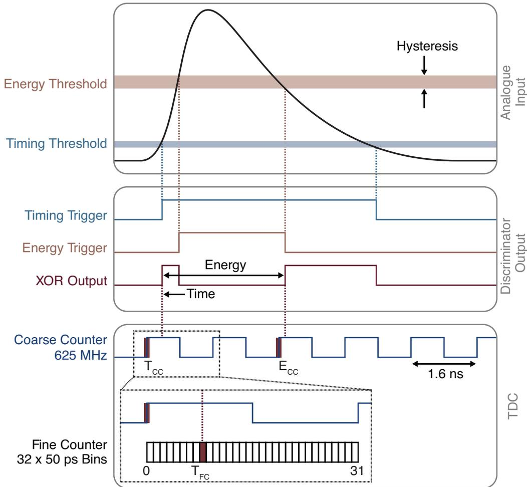
**Figure 5.15** – Operational principle of the MuTRiG ASIC. Two thresholds in fast leading edge discriminators are used to extract time and energy information from the input signal. The outputs from the discriminators are combined such that a single TDC channel can digitize the result and provide time stamps for both measurements.
