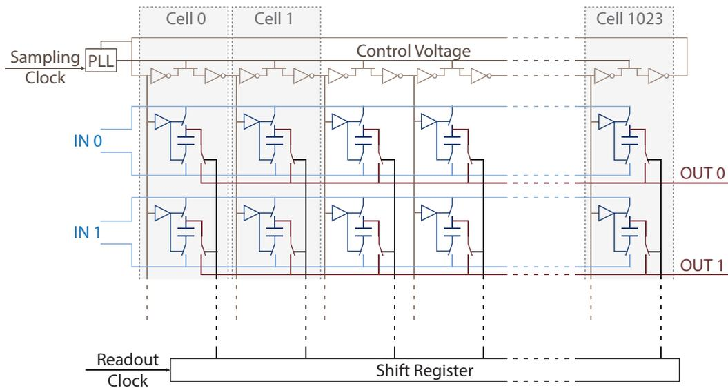
**Figure 5.2** – A control voltage line (—) runs through an inverter chain and activates each cell’s switches (—) to sequentially sample an input signal (—). Once a readout request is made, the sampling stops and a shift register (—) allows consecutive reading (—) of the charge stored in each cell’s capacitor. The sampling frequency is phase locked to a precise external clock for improved stability. The shift register’s clock, on the other hand, is synchronized with an external ADC’s clock.
