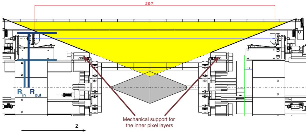
**Figure 8.1** – Geometrical acceptance of the  $\text{Mu3E}$  central detector. A direct line of sight from the outer most pixel sensor in the fourth pixel layer and the center of the target determines the acceptance region. Any non-active components of the SciFi detector should be located outside of this region. The  $R_{in}$  and  $R_{out}$  radii illustrate the dimensions of the geometrical envelop holding the fiber detector.
