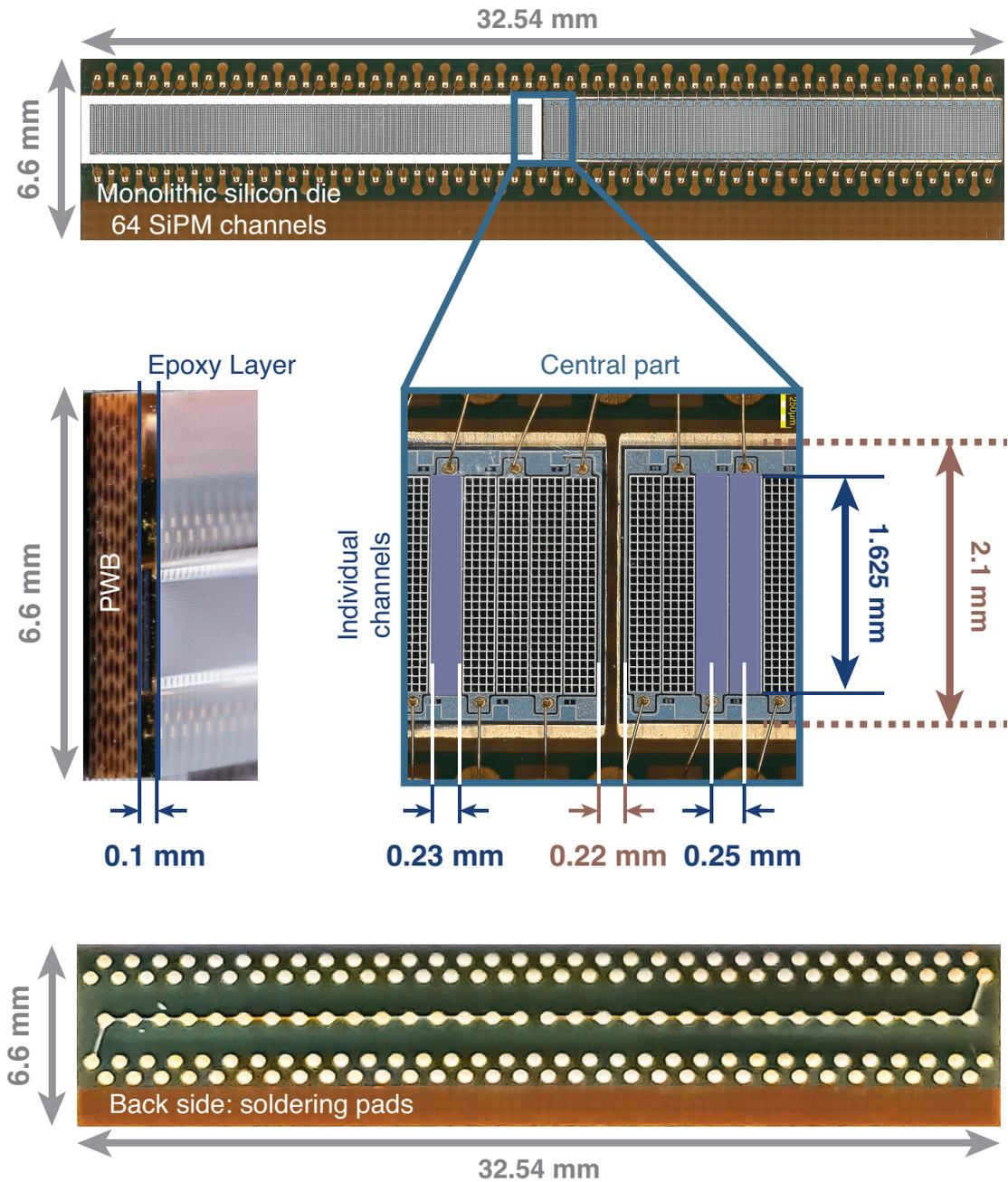
**Figure 4.8** – Picture of a HAMAMATSU S13552 HQR SiPM array. Two such devices are used for the column readout of the SciFi ribbons discussed in chapter 7. The  $M\mu 3E$  experiment will use 24 such sensor to readout 12 fiber ribbons on both sides.
