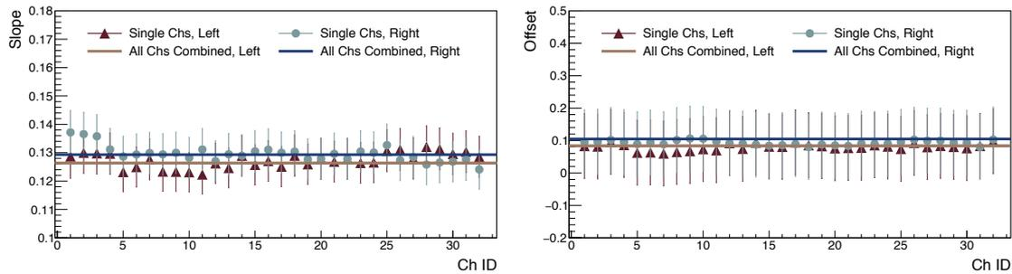
**Figure 7.9** – (Left) Slope  $A_1$  and (Right) offset  $A_0$  coefficients obtained when running the calibration procedure for each channel individually. The straight lines represent the slope and offset extracted when the charge spectra of 32 channels in one SiPM are combined.
