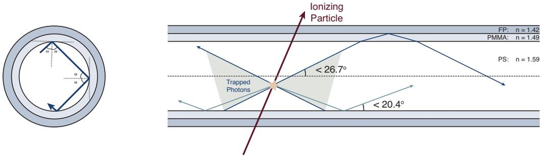
**Figure 3.4** – Illustration of the light trapping in scintillating fibers. (Right) Cross section of a fiber with helical path of the trapped photon. (Left) A longitudinal view of the trapping efficiency for a multiclad fiber. The additional cladding increases the internal reflection angle.
