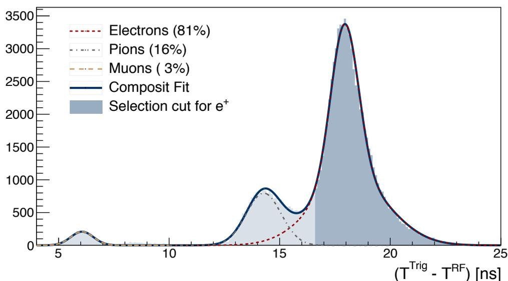
**Figure 7.2** – The  $\pi$ M1 beam consists of pions, muons and electrons in different ratios depending on their momentum. For the 161 MeV/c beam particles the above time of flight between the trigger cross and the  $\pi$ M1 production target is recorded. Particle concentrations are extracted after a composite fit of four Gaussian functions. The shaded area represent the cut applied to select only electrons.
