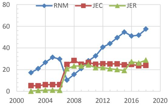
**Fig. 4:** Activity concentration of  $^3\text{H}$  (in GBq/kg) in the SINQ  $\text{D}_2\text{O}$  cooling loops as function of operational year. The „jumps“ in  $^3\text{H}$  concentration for year 2007 and 2016 are due to intentional mixing of heavy water between the circuits [3].
