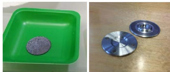
**Fig. 2:** Pressed  $\text{Nd}_2\text{O}_3$ /Graphite pellet with clearly visible heterogenous structure (left). The opened "coin" irradiation target holder (right, courtesy of AEC-LHEP, Univ. Bern).
