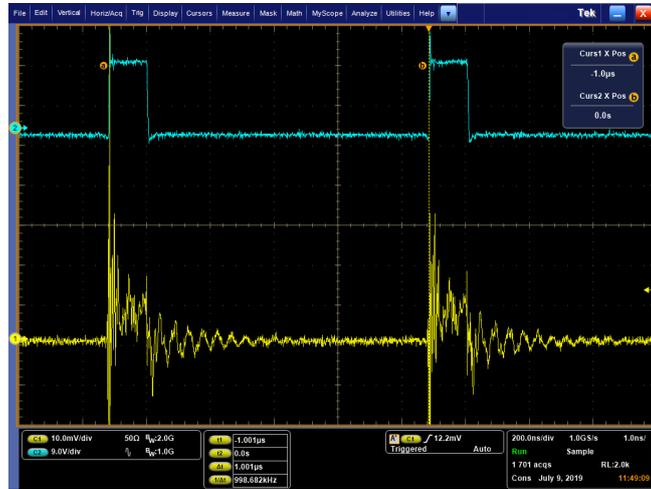
Figure 6.4.: Time domain signal of the radiated noise and the inductor voltage with  $V_{in} = 18 \text{ V}$  and  $V_o = 1.8 \text{ V}$ .
