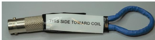
Figure 4.6.: The magnetic near field probe used for the noise measurements.
