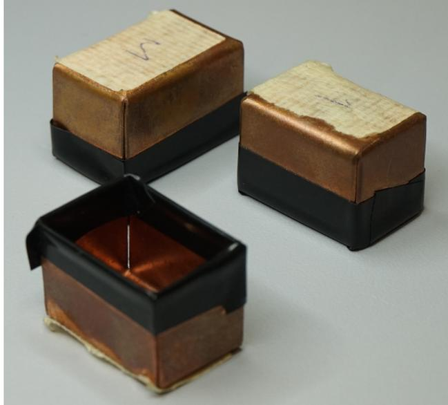
Figure 5.1.: The three copper boxes used as shielding for the frontend board.
