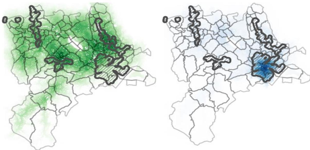
*Figure 5: Spatial distribution of agricultural (left) and non-agricultural (right) biomass in the canton Lucerne. The areas surrounded by a thick grey line are those equipped with a public gas grid. Biogas plants cannot be installed outside that region, as they would have nowhere to sell their products to.*
