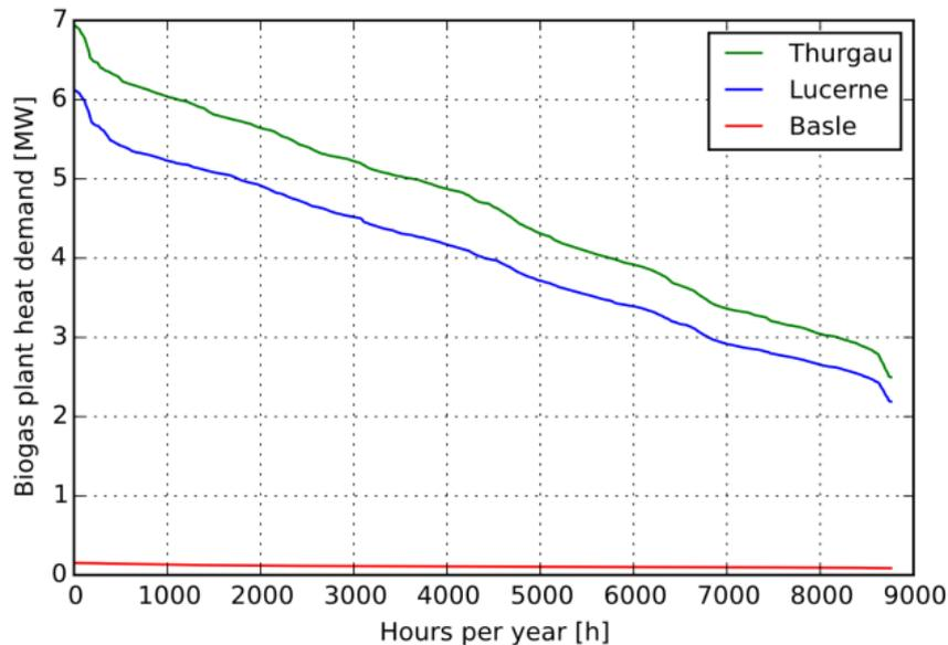
Figure 29: Biogas production plant heat demand duration curves of the case study regions. The heat demand of all biogas plants in a region is summed up.
