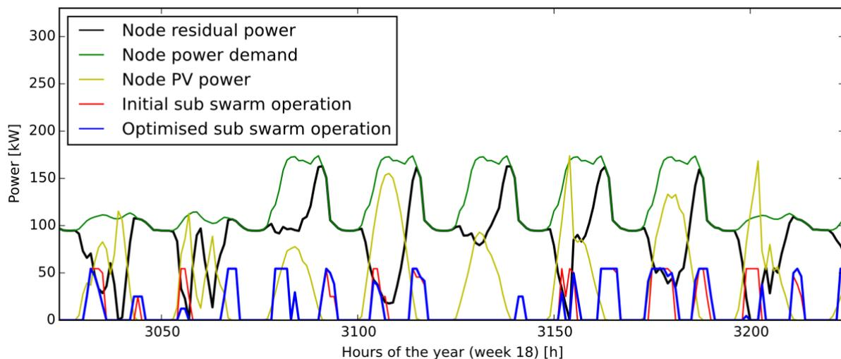
*Figure 18: Example of redispatching of 8 units (3.6, 3.9, 4.1, 4.4, 4.4, 4.5, 4.5, 25 kWel) connected to a common grid node in the canton Lucerne. In essence, an additional, supervisory controller rearranges production so that the swarm never produces more power than is locally consumed. This reduces the annual profits over the whole swarm by merely 0.1‰.*
