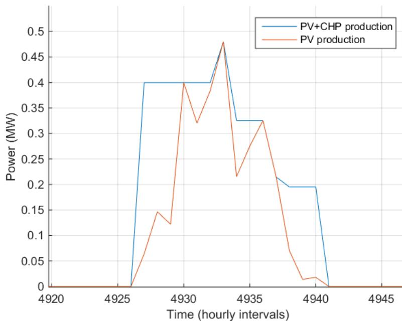
Figure 59: PV and combined PV+CHP generation for Basel City district grid with intermediate PV penetration on July 25<sup>th</sup>
