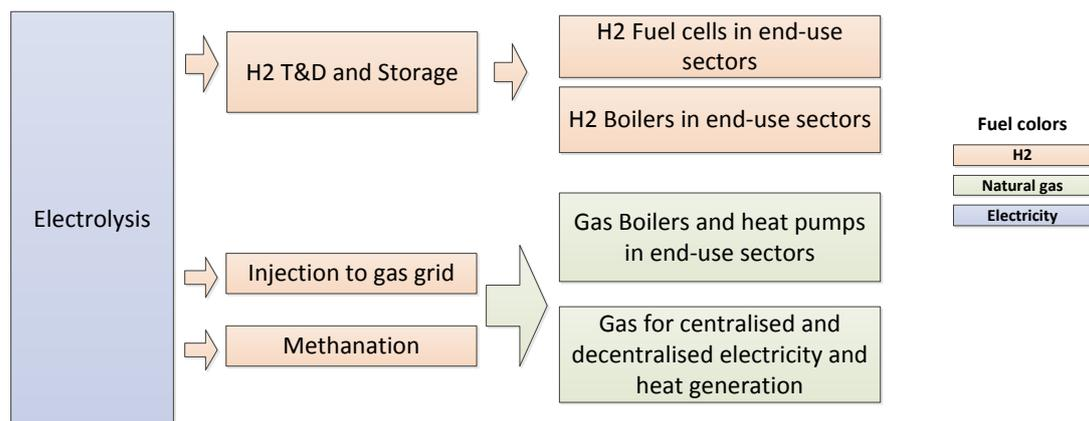
Figure 110: Power-to-gas pathways in STEM-HE model.
