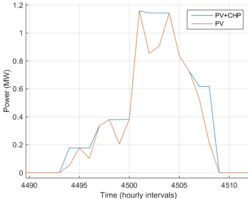
Figure 64: PV and combined PV+CHP generation for Bùrglen (TG) grid with low PV penetration on July 7<sup>th</sup>
