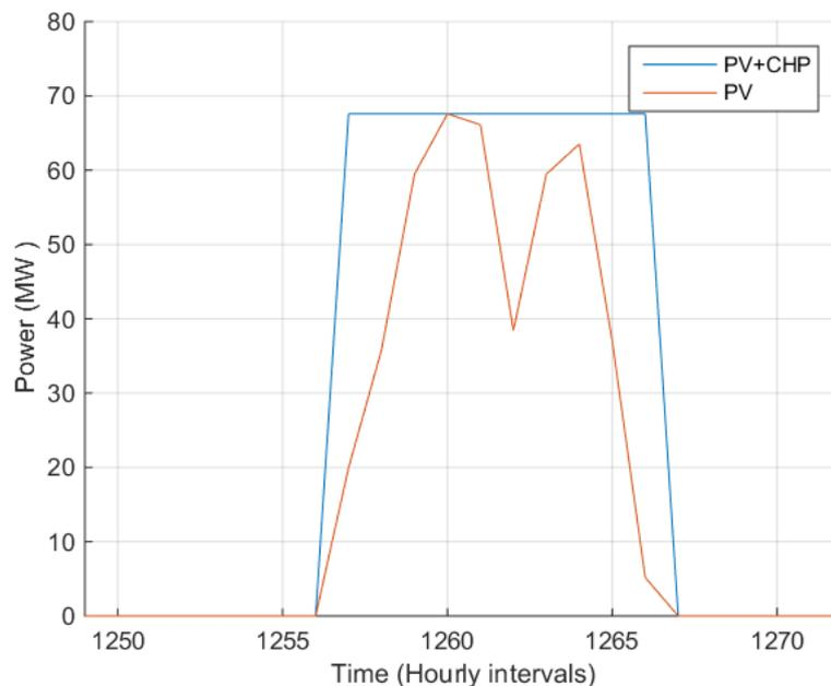
Figure 53: PV and combined PV+CHP generation in CKW grid (Swarm5) with intermediate PV penetration on February 21<sup>st</sup>
