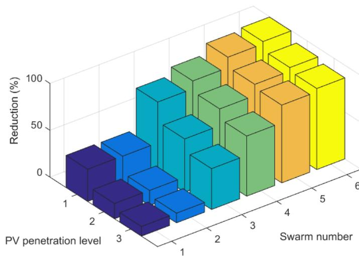
Figure 58: Average yearly percentage reduction between  $\sigma_p$  and  $\sigma_{pc}$  in EWL grid (PV penetration levels 1, 2, 3 correspond to low, intermediate and high scenarios respectively)
