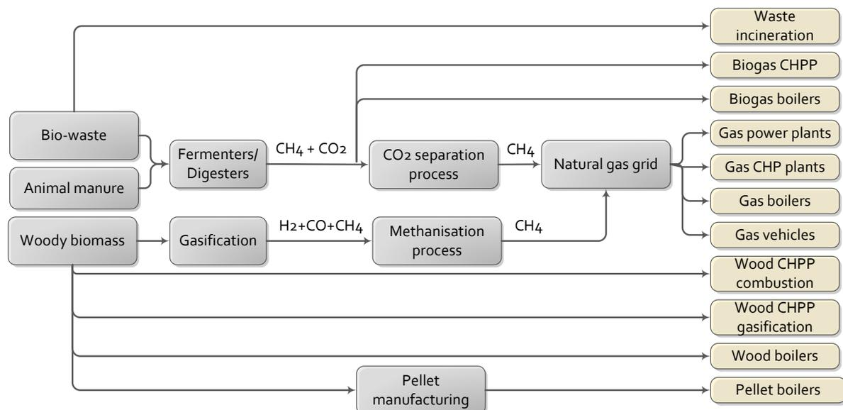
Figure 108: Biogas production and use pathways.
