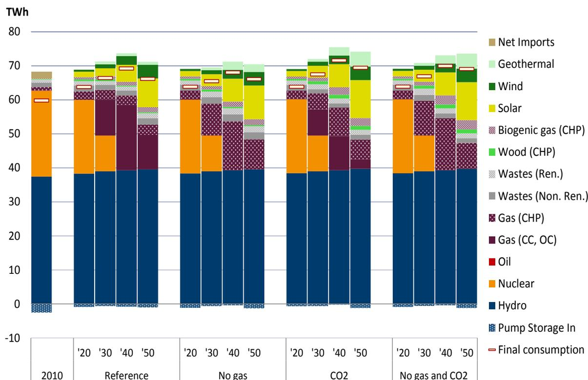
Gas CC=gas turbine combined cycle; Gas OC=gas turbine open cycle; Wastes (Non. Ren.)=non-renewable waste treatment plants (KVA/ARA) ; Wastes (Ren.)=renewable waste treatment plants (KVA/ARA); Wood (CHP) = CHP units using wood on-site (combustion or gasification); Biogenic gas (CHP) = CHP units using biogas or bio-methane from gas grid
