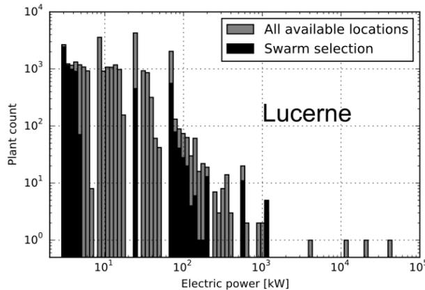
Figure 36: Plant selection for case study region Lucerne (692 GWh biomethane) including grid constraints in the sense that the nominal plant power per node does not exceed the node demand peak.
