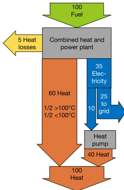
Figure 22: General application of CHP plants for power generation on demand instead a conventional gas boiler heating systems. The same amount of heat is generated with a local or remote heat pump fed via the electricity grid and 25% of quasi “CO<sub>2</sub>-free” electricity is provided.
