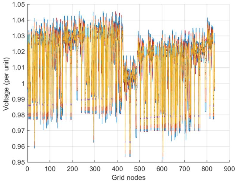
Figure 55: Voltages in the EWL grid (Swarm2) with high PV penetration on June 10<sup>th</sup> (for each node the hourly time series of 24 associated voltages is featured)
