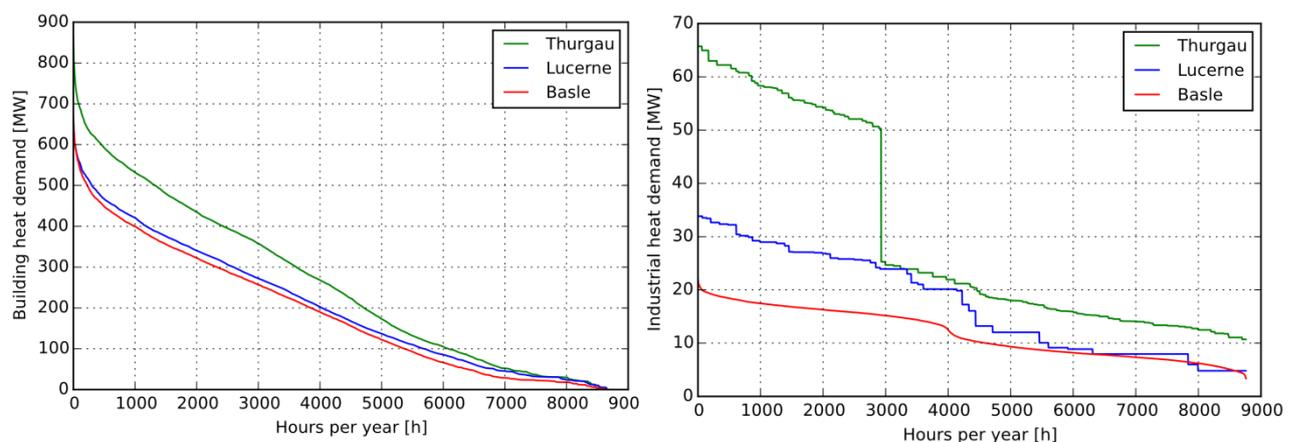
Figure 4: Heat demand load-duration curves from residential (left) and industrial (right) buildings in Thurgau, Lucerne and Basle. The plots are shown in absolute units [MW] to highlight the diverging properties of the three regions. The sudden jump on the right is due to the seasonal operation of one particularly large industrial plant in the canton of Thurgau.
