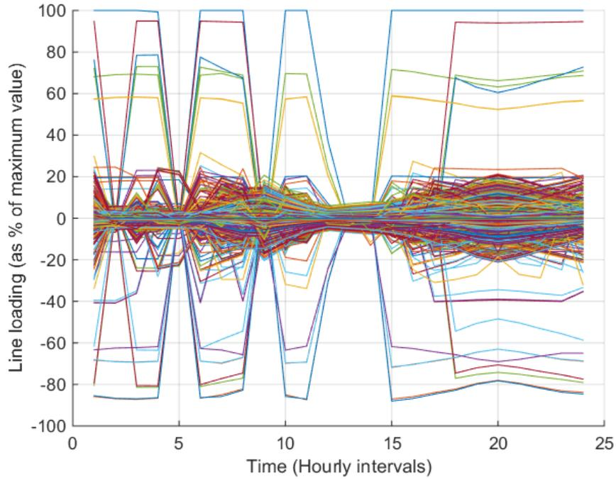
Figure 54: Line loading in the CKW grid (Swarm4) with intermediate PV penetration on January 4<sup>th</sup>
