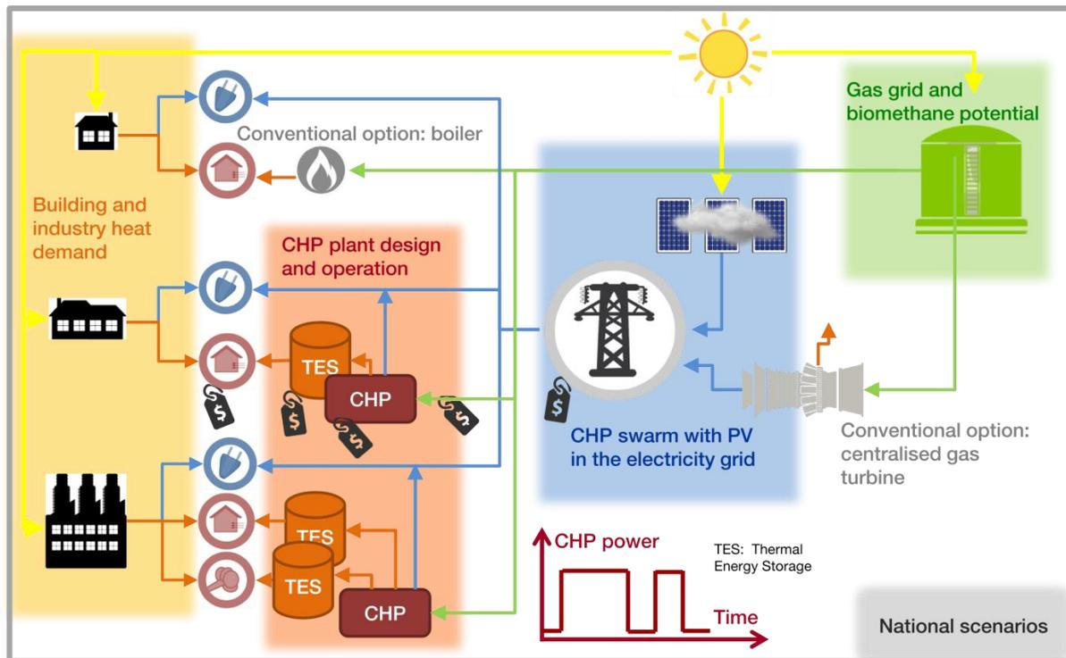
Figure 3: Schema of the system studied within CHPswarm: a building-wise distributed demand for heat and power is to be met by a swarm of CHPPs. To that end, suitable buildings have to be selected, and the CHPP designs adjusted for the specific locations. The production is modulated according to economic considerations. The swarm-size is limited by the biomethane potential. Finally the grid-impact is analysed.
