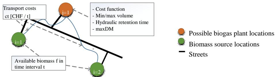
Figure 41: Overview of input parameter used for biogas plant location optimization
