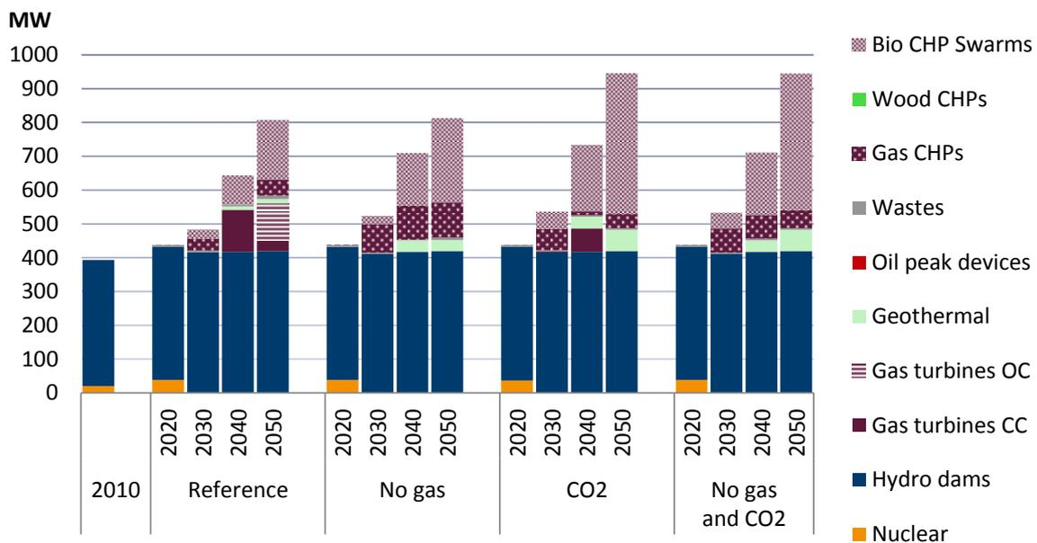
Gas turbines CC=gas turbine combined cycle; Gas turbines OC=gas turbine open cycle; Wastes=renewable and non-renewable waste treatment plants (KVA/ARA) ; Gas CHPs = natural gas-fired CHPP; Wood CHPs = CHP units using wood on-site (combustion or gasification); Bio CHP Swarms = CHP units fuelled by bio-methane/biogas and operate as swarm
