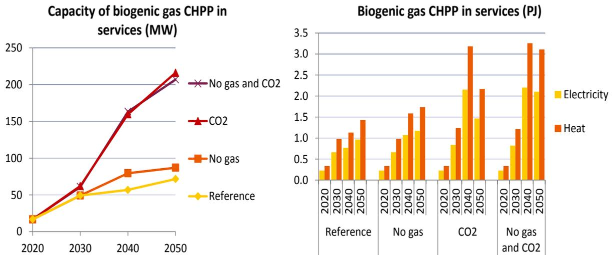
Figure 88: Installed capacity and production from biogenic gas CHP plants in services.
