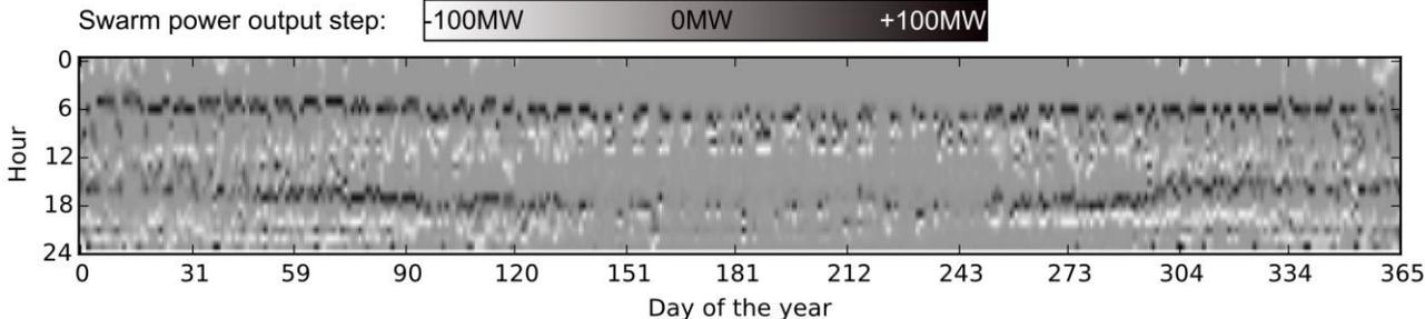
Figure 39: Aggregated power output of all plants of the swarm in Lucerne over 8760 h
