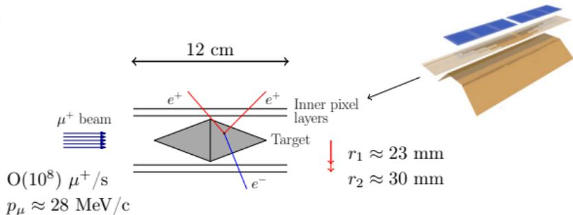
Muons stop and decay on target:
