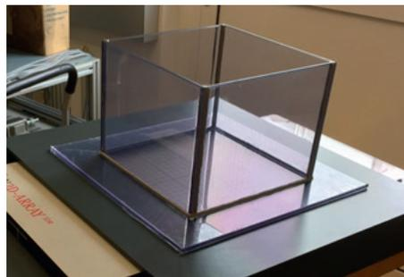
Figure 2: A 2D ionization chamber array mounted on a moving platform placed under a “bridge” which holds a water phantom.
