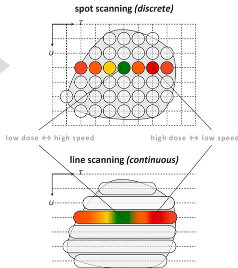
**Figure 1:** Schematic comparison of spot and line scanning. In the former delivery mode, protons are irradiated to positions on a discretized grid; in the latter mode, the proton beam is steered continuously along straight lines without being turned off in between.
