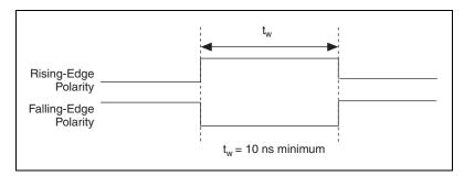
Figure 4-34. GPCTR1\_OUT Signal Timing
