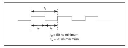
Figure 4-29. GPCTR0\_SOURCE Signal Timing
