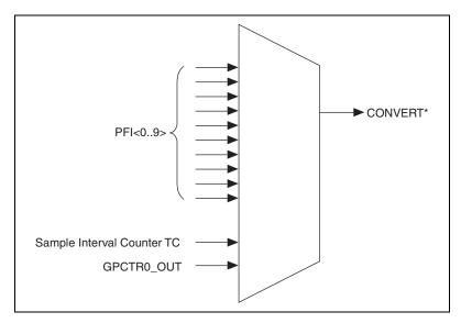
Figure 3-2. CONVERT\* Signal Routing
