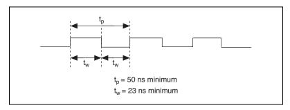
Figure 4-32. GPCTR1\_SOURCE Signal Timing
