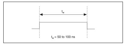
Figure 4-25. WFTRIG Output Signal Timing
