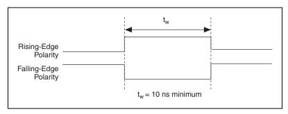
Figure 4-30. GPCTRO\_GATE Signal Timing in Edge-Detection Mode
