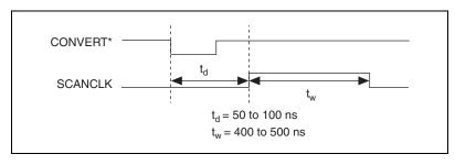
Figure 4-22. SCANCLK Signal Timing
