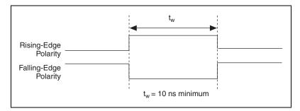
Figure 4-19. CONVERT\* Input Signal Timing
