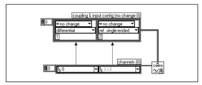
Figure C-1. Configuring Channels to Acquire in Different Modes in LabVIEW
