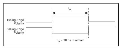
Figure 4-13. TRIG1 Input Signal Timing
