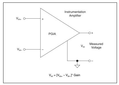
Figure 4-2. Programmable Gain Instrumentation Amplifier (PGIA)
