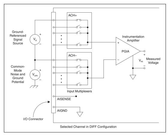
Figure 4-4. Differential Input Connections for Ground-Referenced Signals
