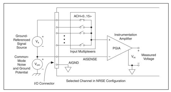
Figure 4-7. Single-Ended Input Connections for Ground-Referenced Signals
