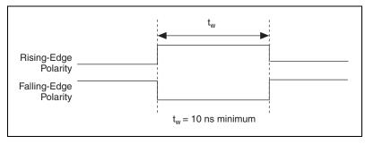
Figure 4-33. GPCTR1\_GATE Signal Timing in Edge-Detection Mode
