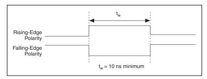
Figure 4-15. TRIG2 Input Signal Timing
