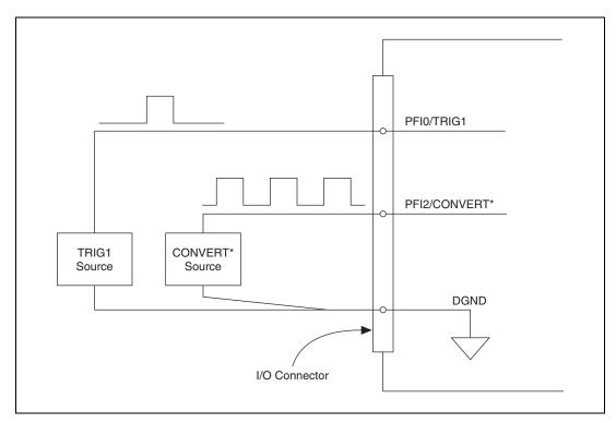
Figure 4-10. Timing I/O Connections
