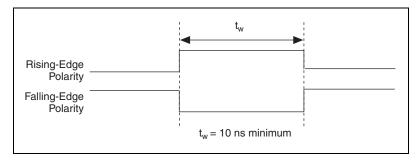
Figure 4-17. STARTSCAN Input Signal Timing
