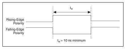
Figure 4-24. WFTRIG Input Signal Timing
