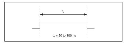
Figure 4-14. TRIG1 Output Signal Timing
