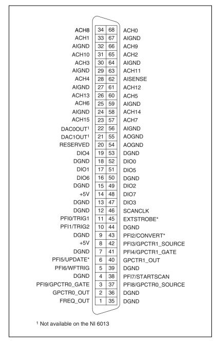
Figure B-1. 68-Pin Connector Pin Assignments
