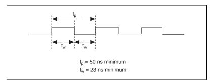
Figure 4-21. SISOURCE Signal Timing
