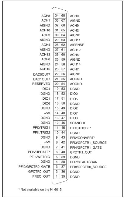
Figure 4-1. I/O Connector Pin Assignment for the NI 6013/6014
