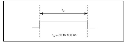
Figure 4-16. TRIG2 Output Signal Timing
