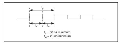
Figure 4-28. UISOURCE Signal Timing
