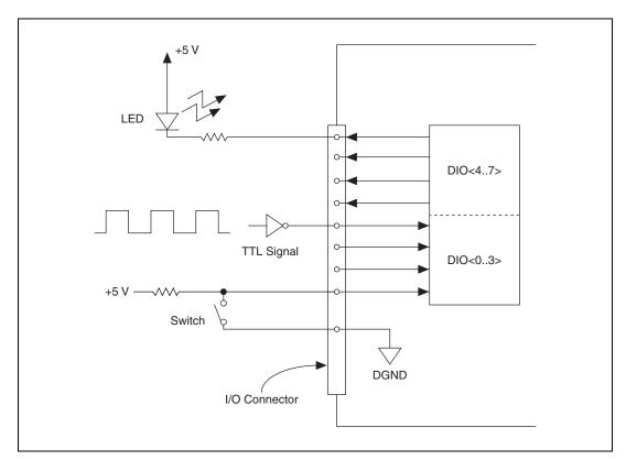
Figure 4-9. Digital I/O Connections
