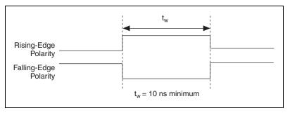
Figure 4-26. UPDATE\* Input Signal Timing
