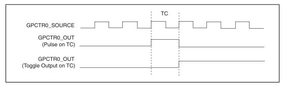
Figure 4-31. GPCTR0\_OUT Signal Timing
