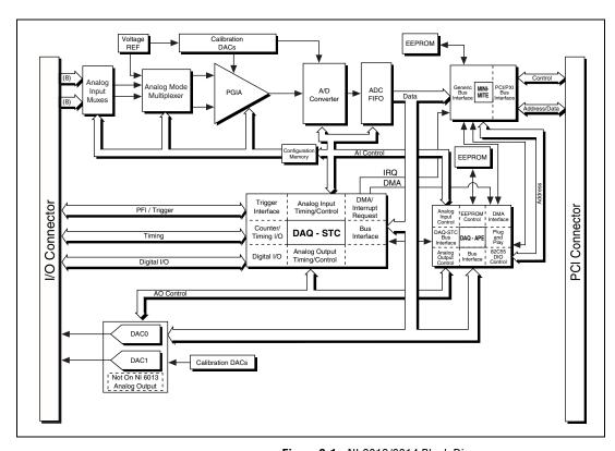
Figure 3-1. NI 6013/6014 Block Diagram
