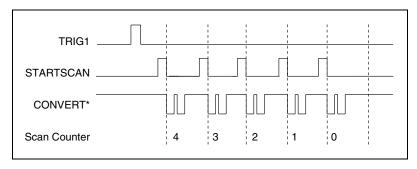
Figure 4-11. Typical Posttriggered Acquisition
