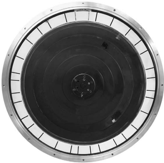
Fig. 2. Picture of the chopper disc. The 32 slits are arranged in four identical sequences with pseudo-random distribution.
