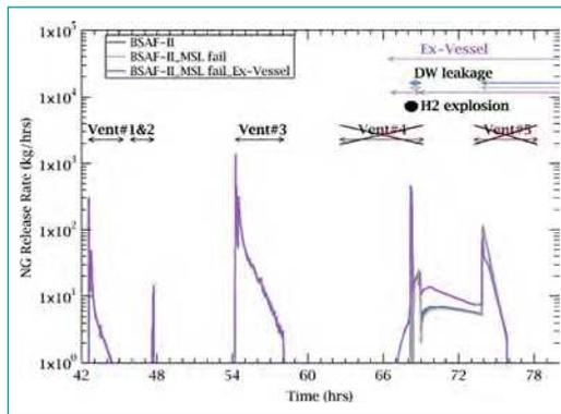
head flange. These results would reinforce the assumption of DW leakage before the H<sub>2</sub> explosion made during the BSAF phase 1.
