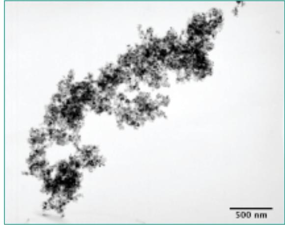
Fig. 4: Agglomerate TiO<sub>2</sub> particles used in ARTIST tests (picture: Lind et al., 2008).
