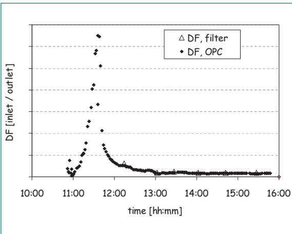
Fig. 5: Decontamination factor in the single tube in the test with high concentration of spherical SiO<sub>2</sub> particles was dynamic with time (picture: Lind et al., 2008).
