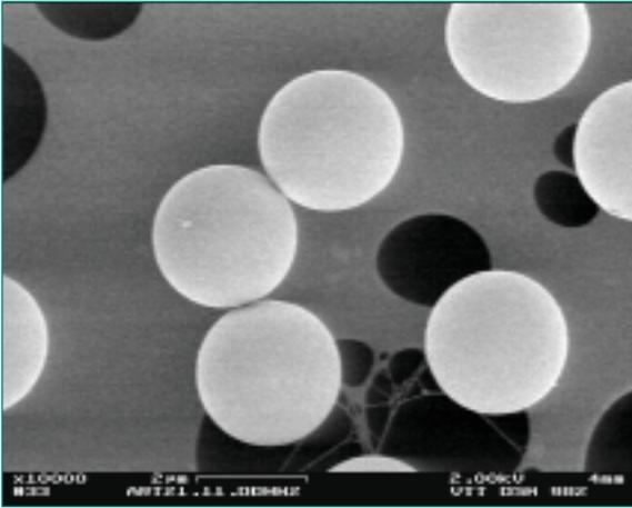
Fig. 3: Spherical, monodisperse SiO<sub>2</sub> particles used in ARTIST tests (picture: Lind et al., 2008).
