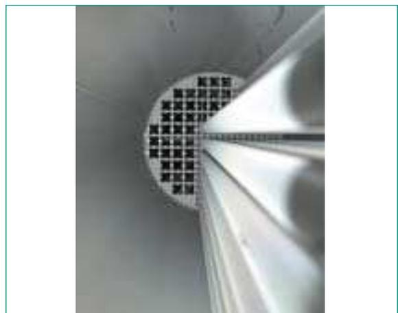
Fig. 8: A photograph of the ARTIST far field facility after a test with SiO<sub>2</sub> aerosol particles showing a thin layer of particle deposit on the tube and shroud surfaces (picture: Lind et al., 2008).
