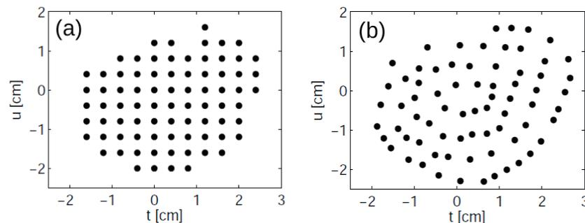
**Figure 1** Single energy layer for standard grid (a) and contour spot placement (b).
