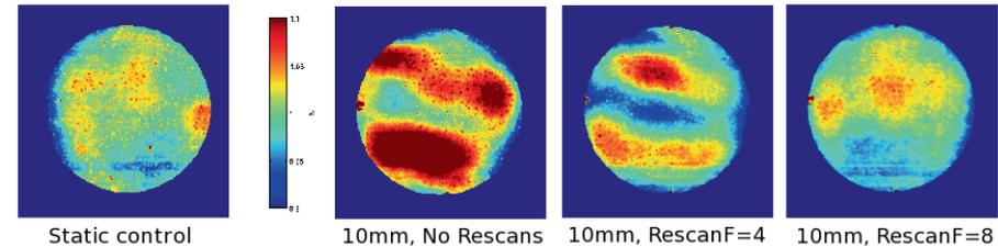
**Figure 2** Central plane of target in static, moving with 10 mm sine motion, with variable rescanning. Colour scales shows %Dose normalized to the mean dose of the static control film, ranging from blue = 90 % to red = 110 %.
