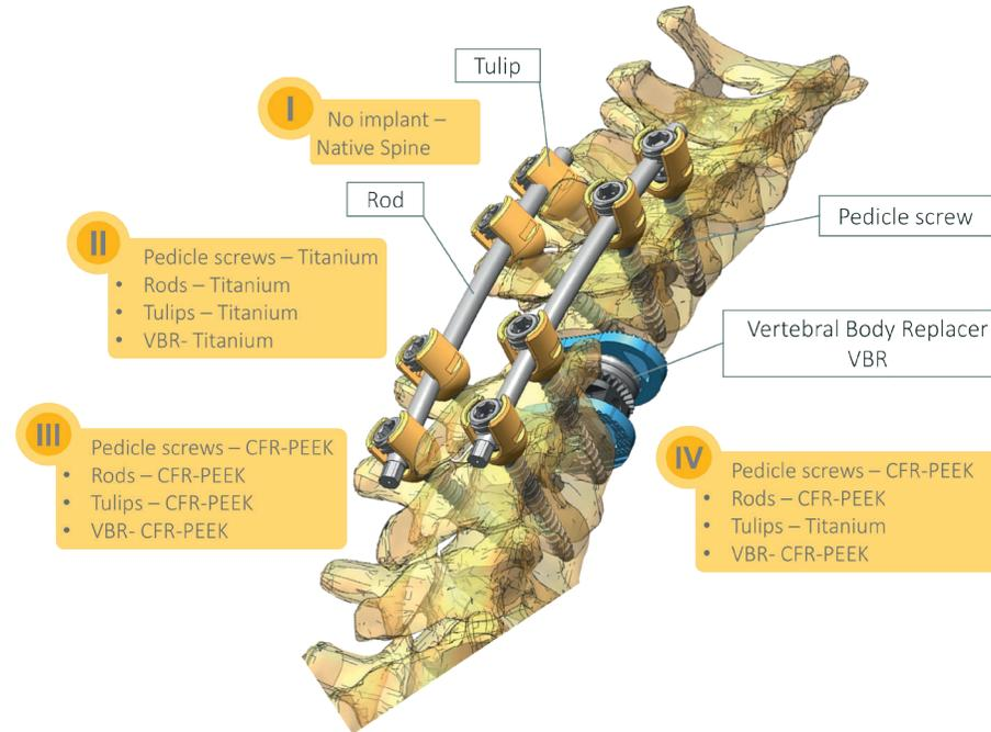
Design schematic of the interchangeable insert of the phantom. The 4 different inserts exist of: A native spine (case I), a full titanium implant (case II), an implant completely out of CFR-PEEK (case III) and a hybrid implant where the tulips are made of titanium (case IV).
