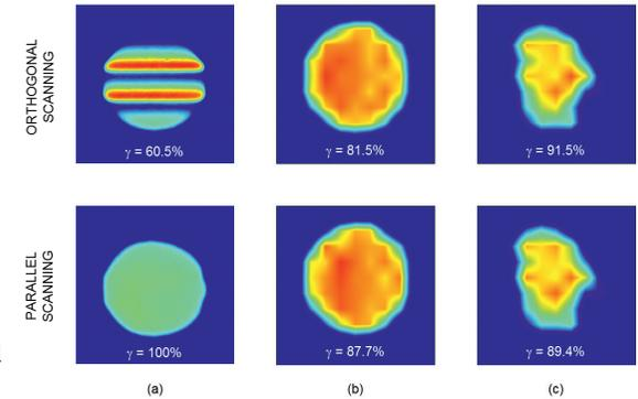
**Figure 2:** measured dose distributions scanning under similar experimental settings for single energy layer (a), spherical target (b) and patient field (c).  $\gamma$ -scores calculated at 3%/3mm for all pixels above 5% of prescribed dose.
