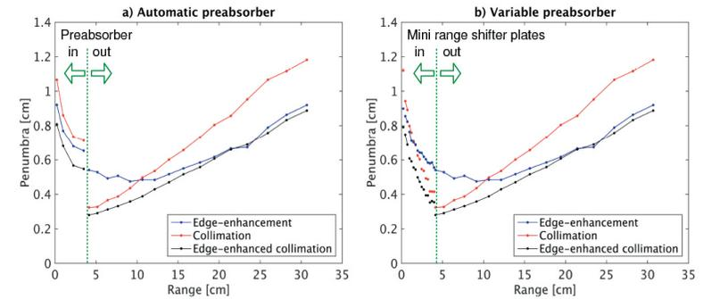
**Figure 2:** Penumbra at the Bragg peak for edge-enhancement (blue), collimation (red) and edge-enhanced collimation (black). The initial beam energy is reduced using (a) a pre-absorber, which is inserted for the delivery of low energy Bragg peaks only (automatic pre-absorber) or (b) a combination of up to eight mini range shifter plates (variable pre-absorber).
