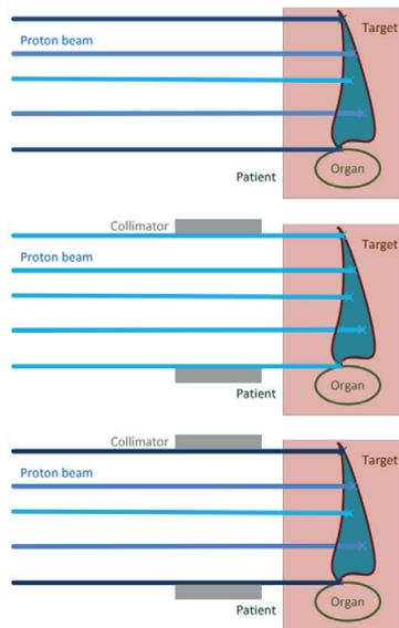
**Figure 1:** To achieve a sharp lateral falloff, (a) the weights of the uncollimated pencil beams are optimized, darker lines represent spots with more protons (edgeenhancement), (b) uniform weighted pencil beams are collimated (collimation) or (c) the weights of the collimated pencil beams are optimized (edgeenhanced collimation).
