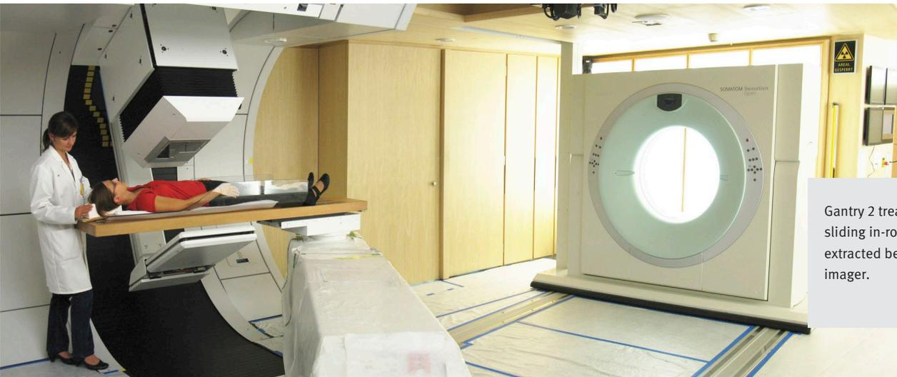
Gantry 2 treatment room with sliding in-room CT and extracted beam's-eye-view imager.
