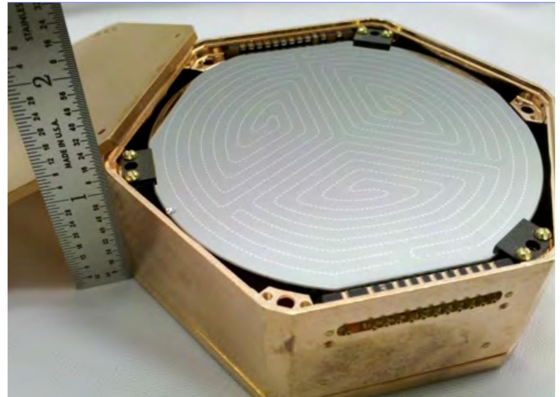
Five super-towers had been installed at Soudan, each with 3 new, iZIP detectors, of 650 g
