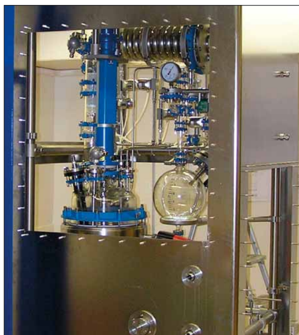
Figure 1: Installation of the distillation column in its alpha-containment.
