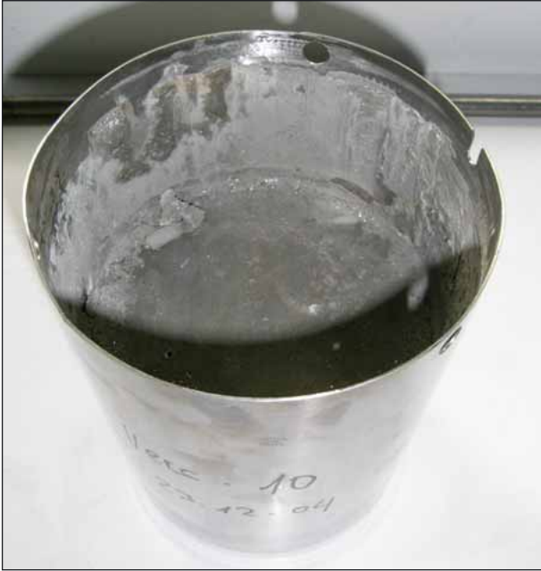
Figure 2: Steel casing containing a cement brick (test).
