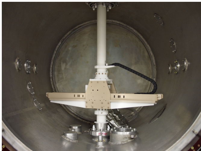
Figure 6.1: Mapping device located inside the vacuum tank.
