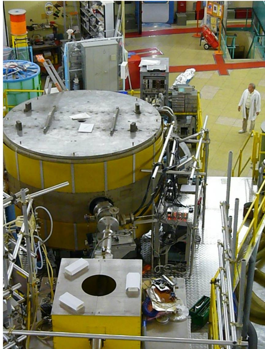
Direct measurement of sensitivity of EDM spectrometer with UCN density 3-4 ucn/cm<sup>3</sup> (MAM position) with electric field 10 kV/cm and T(hold) = 65 s
