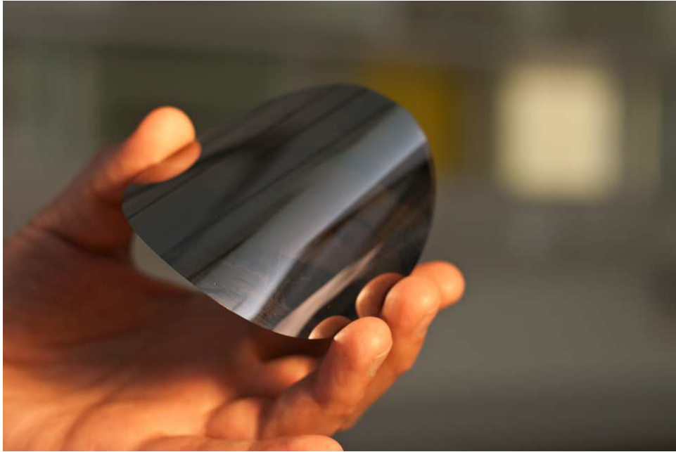
Figure 10.19: A 50 \mu\text{m} thin silicon wafer.
