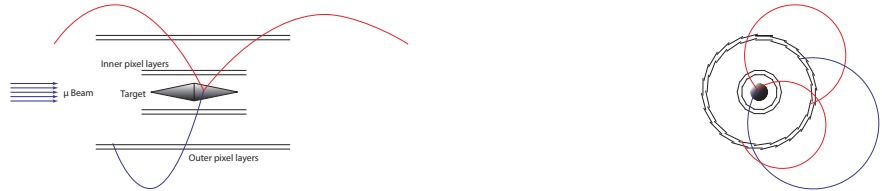
Figure 6.7: Minimum detector configuration for early commissioning with central silicon only (phase IA).
