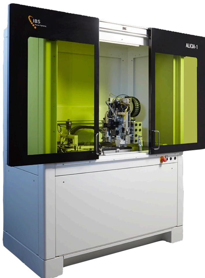
The modules are being assembled using a custom machine (**ALICIA**), which aligns the chips into the HIC positions (position accuracy  $\pm 5 \mu\text{m}$ ) and provides the possibility to probe the chips and to do a fully automatic visual inspection.
