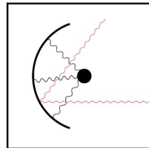
MADMAX: combines the dish antenna with a tunable resonating structure out of dielectric disks to boost the axion-photon conversion probability.
