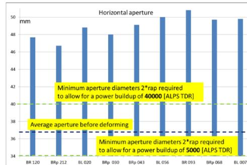
Figure 6.2: Horizontal aperture of HERA dipoles after straightening
