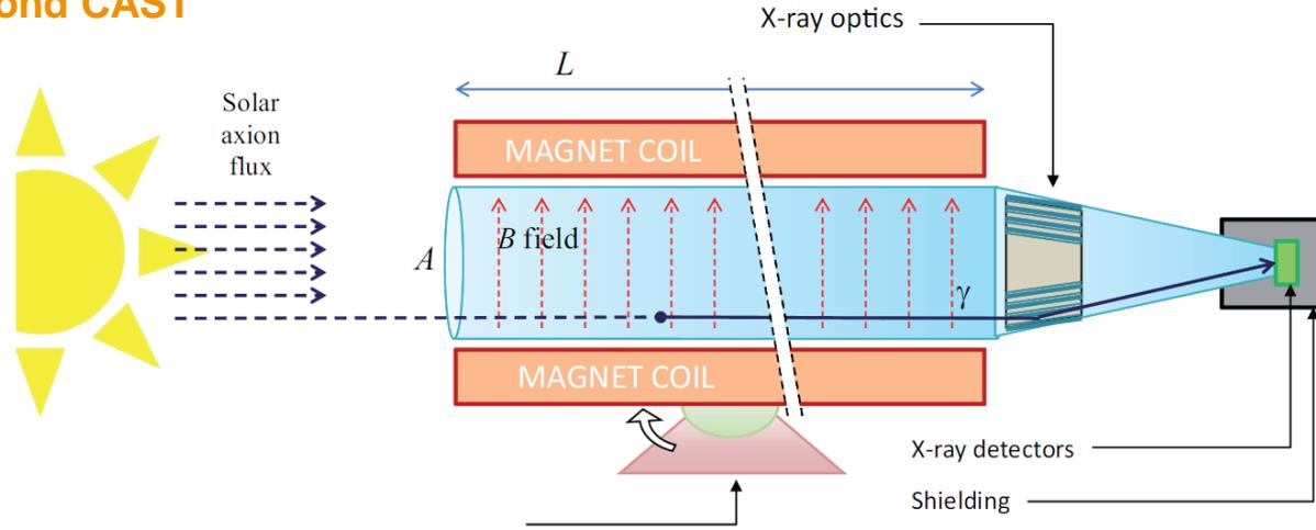
$$g_{a\gamma}^4 \propto \underbrace{b^{1/2} \epsilon^{-1}}_{\text{detectors}} \times \underbrace{a^{1/2} \epsilon_o^{-1}}_{\text{optics}} \times \underbrace{(BL)^{-2} A^{-1}}_{\text{magnet}} \times \underbrace{t^{-1/2}}_{\text{exposure}}$$
