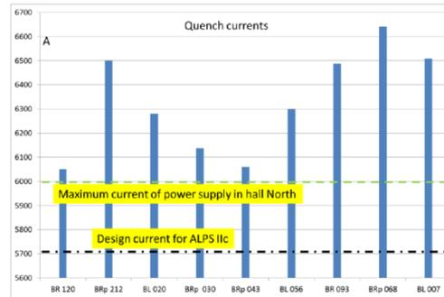
Figure 6.1: Obtained quench currents of straightened HERA dipoles
