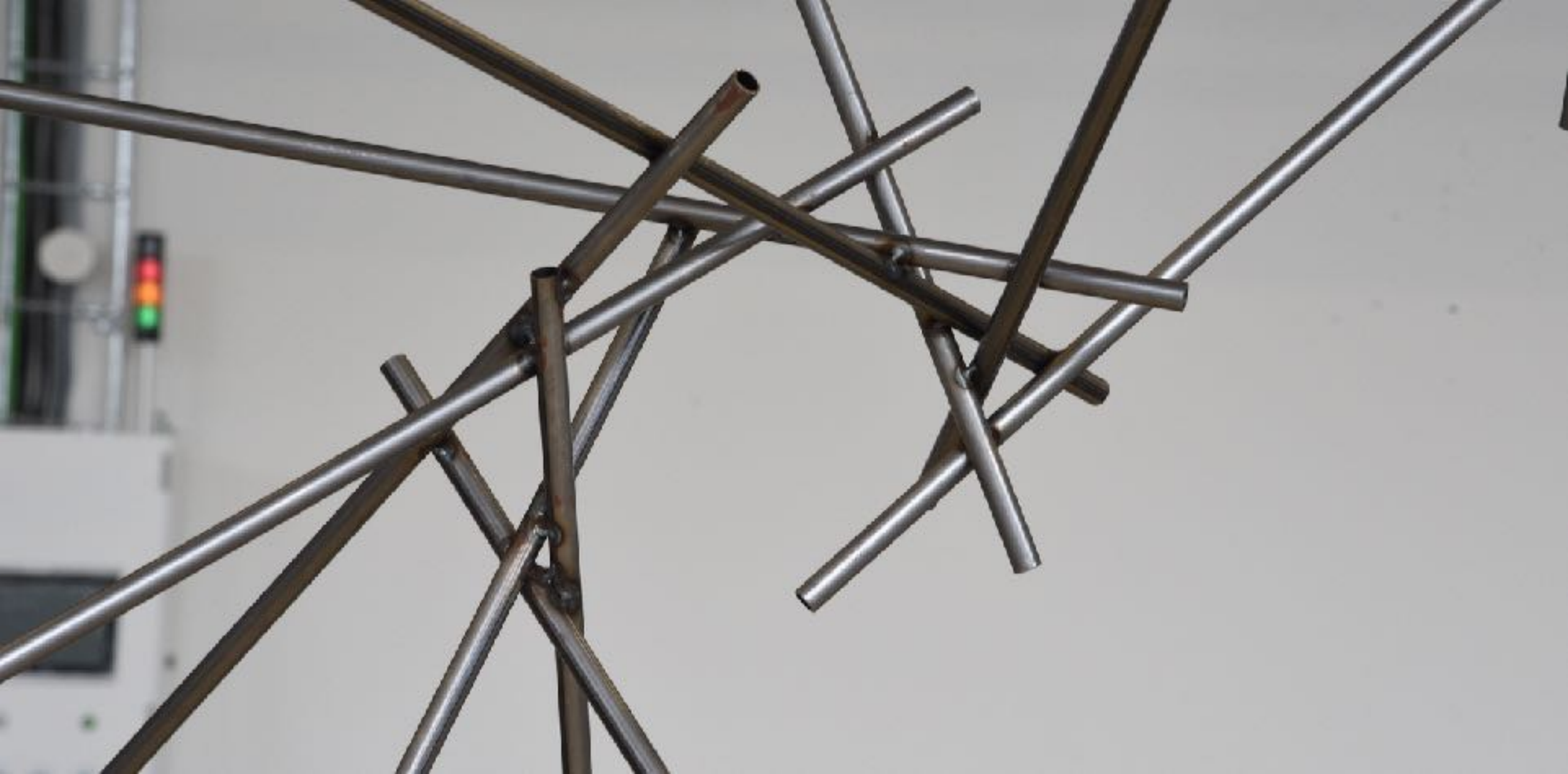
Steel Welded Spatial Assembly NCCR Digital Fabrication
