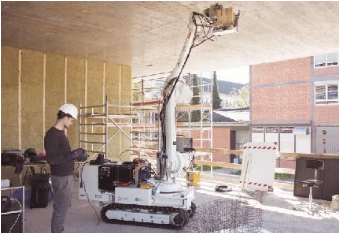
Left: In situ Fabricator test on NEST, Right: Robotic joining of timber plates
