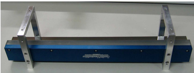
Figure 11.7: Single guide element (half a guide section). The blue part is an L-shaped Al bar on which the glass substrates are screwed. The Al frames are for mounting the elements on the support and alignment system.
