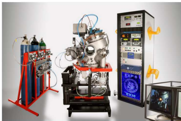
Figure 12.8: Photo of the sputtering system with the sputtering chamber in the middle, the gas rack on the left, and the electronic rack and the computer on the right. (Source:[35])
