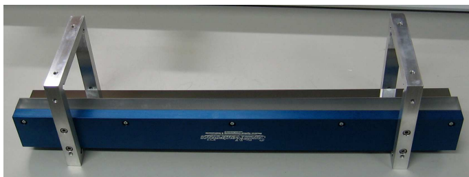
Figure 12.6: Guide support with 2 guide elements mounted. Shown is the second guide of the Selene set-up, reflecting left and downwards. The guides are not yet adjusted, the knife blade slit is missing.
