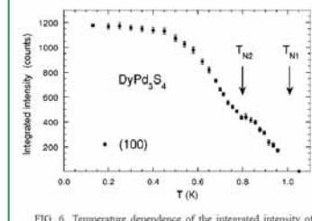
FIG. 6. Temperature dependence of the integrated intensity of the magnetic (100) peak, determined by neutron diffraction.
