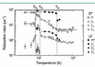
FIG. 1. Temperature dependences of the muon spin relaxation rates. The zero (ZF) and longitudinal field (LF) experiments are shown by open and filled symbols, respectively. Anomalies at  $T_O$ ,  $T_{N_1}$ , and  $T_{N_2}$  are signatures of the quadrupolar and the magnetic ordering phenomena.
