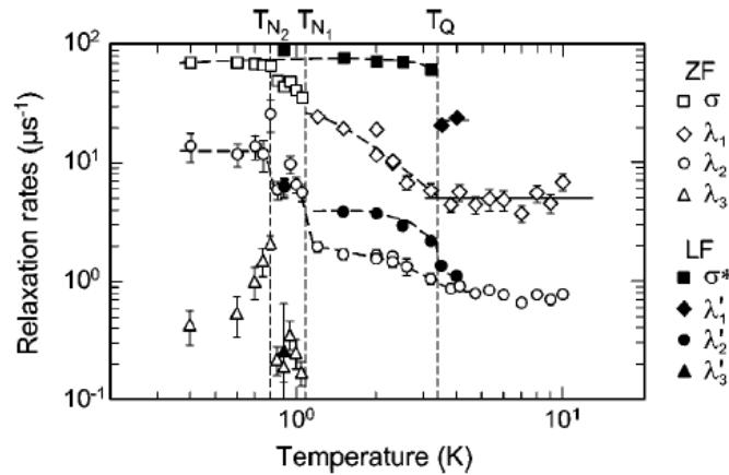
FIG. 1. Temperature dependences of the muon spin relaxation rates. The zero (ZF) and longitudinal field (LF) experiments are shown by open and filled symbols, respectively. Anomalies at  $T_Q$ ,  $T_{N1}$ , and  $T_{N2}$  are signatures of the quadrupolar and the magnetic ordering phenomena.
