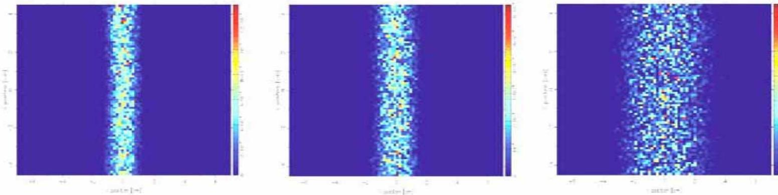
**Figure 1:** PSD images of the 9cm-detector for bragg reflections  $35.73^\circ$ ,  $51.42^\circ$  and  $90.2^\circ$
