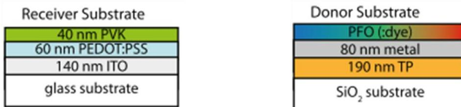
Figure 6: Structures of the receiver and the donor substrates
