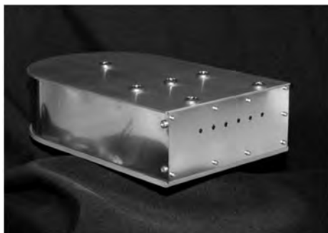
Fig. 25 The ms-LPT after assembly and during tests in vacuum. At right, the operating device is mounted on a torsion pendulum to measure thrust in vacuum (see [4]); used with permission of the American Institute of Physics, copyright 2007.
