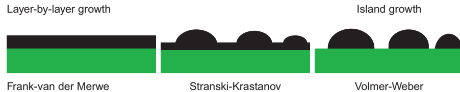
Fig. 5.3 Growth modes. The three growth mode categories are schematically shown. The Frank-van der Merwe growth mode corresponds to a layer-by-layer (2D) growth and the Volmer-Weber to an island (3D) growth. The Stranski-Krastanov growth mode is a mixture of the 2D and 3D growth modes.
