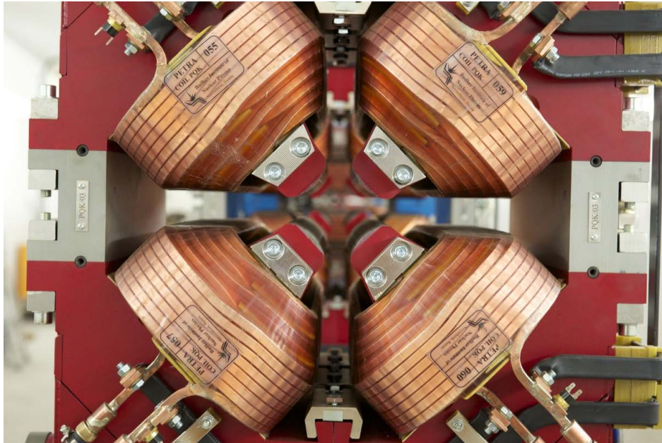
Figure 1.38.: Typical quadrupole magnet.
