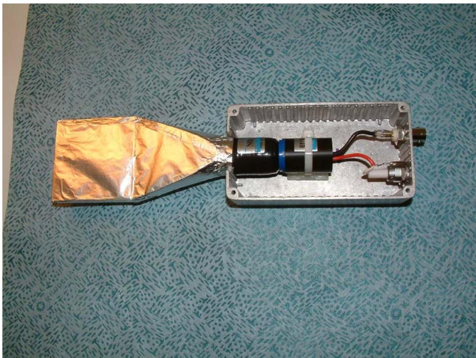
Figure 2. Photograph of the assembled scintillator detector. The scintillator and waveguide shown on the left of the picture are covered in aluminium foil and are connected optically to the PMT (HAMATSU R5505) inside the metal housing.
