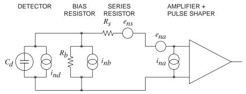
Figure 28.8: Equivalent circuit for noise analysis.
