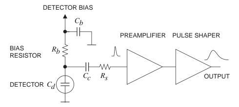
Figure 28.7: Typical detector front-end circuit.
