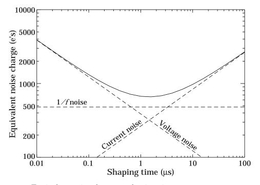
Figure 28.9: Equivalent noise charge vs shaping time.
