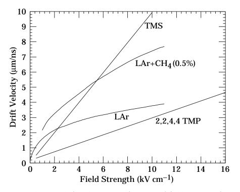
Figure 28.11: Electron drift velocity as a function of field strength for commonly used liquids.
