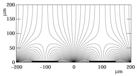
**Figure 28.4:** Electron drift lines in a micro-strip gas chamber with a pitch of  $200 \ \mu m.$
