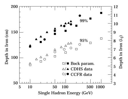
Figure 28.10: Required calorimeter thickness for 95% and 99% hadronic cascade containment in iron, on the basis of data from two large neutrino detectors and the parameterization of Bock et al. [106].
