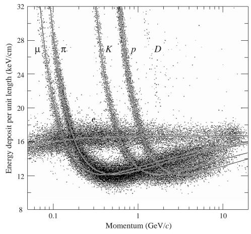
Figure 28.5: PEP4/9-TPC energy-deposit measurements (185 samples @8.5 atm Ar-CH<sub>4</sub> 80–20%) in multihadron events. The electrons reach a Fermi plateau value of 1.4 times the most probably energy deposit at minimum ionization. Muons from pion decays are separated from pions at low momentum;  $\pi/K$  are separated over all momenta except in the cross-over region. (Low-momentum protons and deuterons originate from hadron-nucleus collisions in inner materials such as the beam pipe.)
