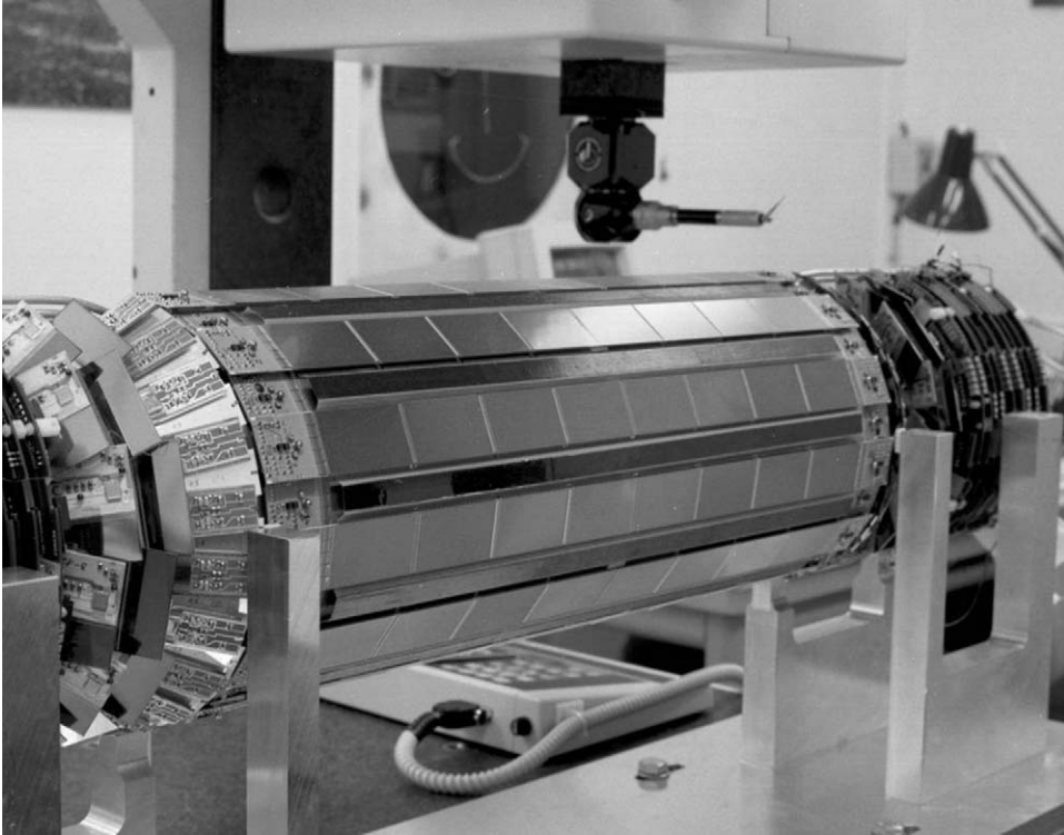
Fig. 8. The latest version of the DELPHI silicon vertex detector at the metrology stand.
