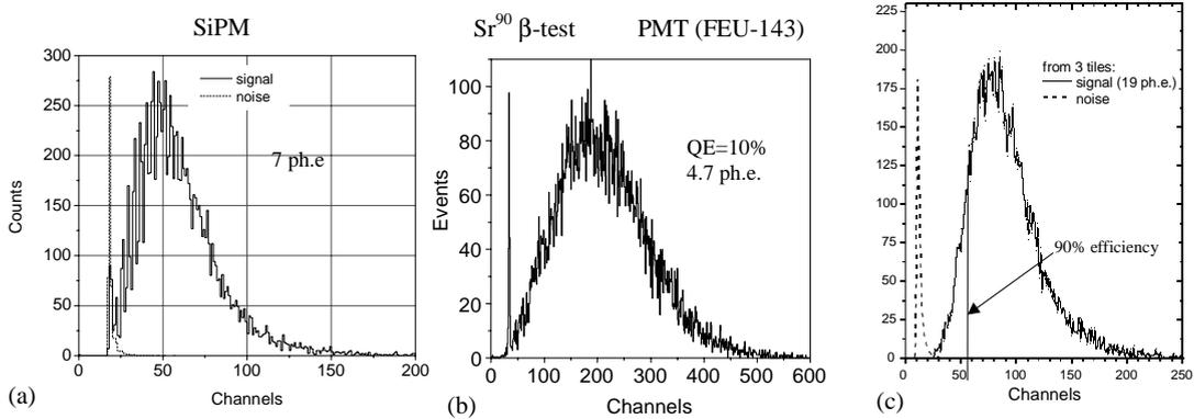
Fig. 4. SiPM application for scintillator and wavelength shifter readout. MIP particle detection is shown using one  $5 \times 5 \times 0.5 \text{ mm}^3$  sci tile and SiPM (a) or PMT (b) and the setup with three cells each consisting of tile + SiPM (c).
