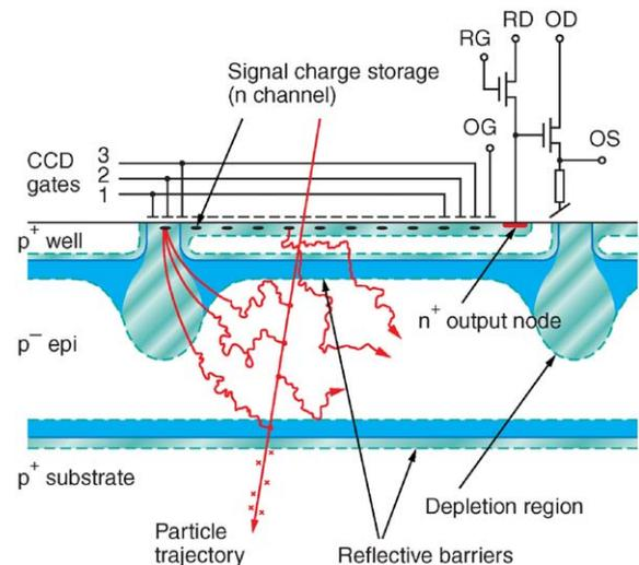
Fig. 3. Sketch of ISIS cross-section (not to scale). Signal charge is reflected from the  $p^-/p^+$  edges above and below the epitaxial layer, so it diffuses within this layer till being collected in the depleted regions beneath the photogates. 10 storage pixels are shown: for the real detector there would be 20.
