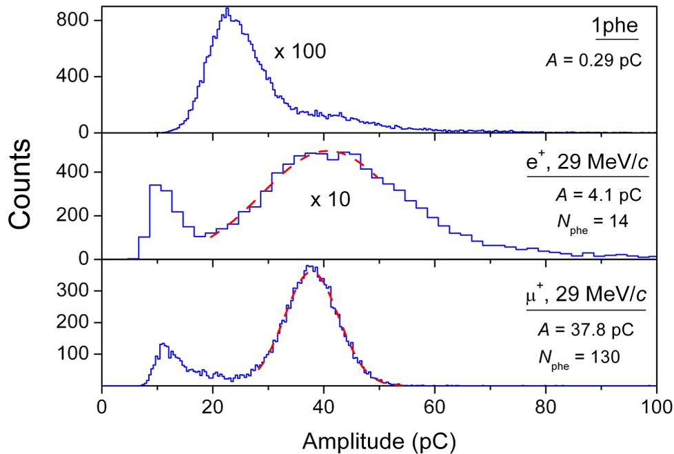
Figure 1: Charge distributions of signals from a detector based on a  $1 \times 1 \text{ mm}^2$  ZS-2mp AMPD with a  $1 \times 1 \times 0.2 \text{ mm}^3$  EJ-230 scintillator. The distributions for 29 MeV/ $c$  positron and muon signals are compared with that for the "dark" (1phe) signals. The values of  $A$  given in the plots are the mean amplitude for 1phe signals, and the most probable amplitudes for  $e^+$  and  $\mu^+$  signals.
