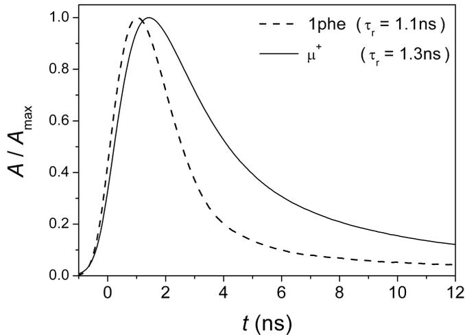
Figure 2: Averaged waveforms (typ. 1000) of 1phe and muon signals.
