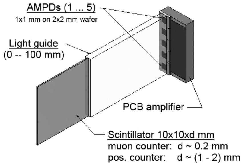
Figure 4: A design concept of a scintillation detector based on an array of AMPDs. The AMPDs are mounted directly on the printed circuit board (PCB) of an amplifier. The linear dimension of the array matches that of the scintillator.
