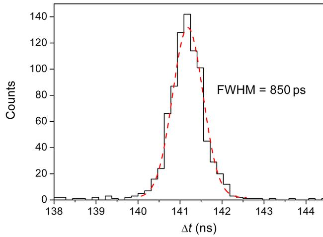
Figure 3: Time resolution of the telescope of two identical detectors (AMPD +  $1 \times 1 \times 0.2 \text{ mm}^3$  EJ-230 scintillator) for registration of electrons from a  $\text{Sr}^{90}$  source.
