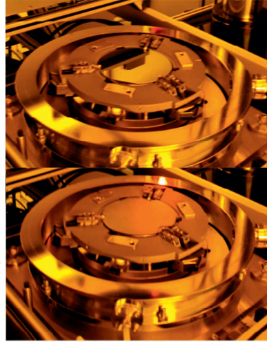
Figure 5.9: Jenoptik HEX03 nanoimprint machine with and integrated adapter for a Süss alignment fixture for an anodic bonder. Alignment is possible by using the appropriate mask aligner.
