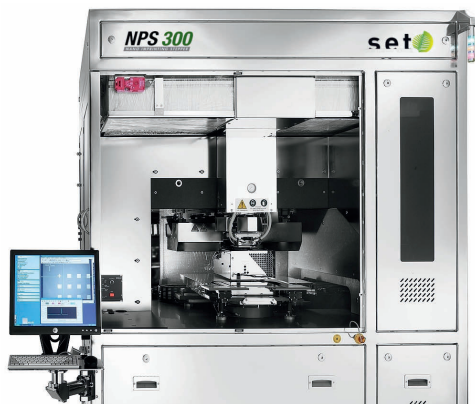
Figures: NPS Step and Stamp machine for thermal and UV NIL used for these experiments (until 2007 SET was part of SÜSS Microtec), installed at VTT (left side), and example (right side) of a 237 consecutive thermal imprints into a 300 nm thick mr-1 7030 film on a 100mm Silicon wafer. Stamp size 4x4mm 2 , micrometer features with sizes of down to 2 μm and height of ~ 200nm. Stamp Temperature:140 °C, substrate temperature 70 °C, cycle time ~ 3 minutes (without collimation and arm movements).
