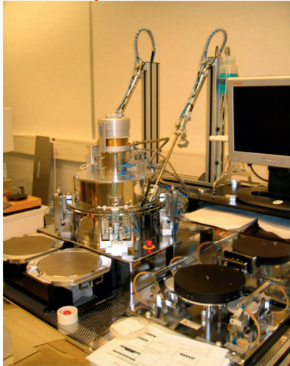
Figure 5.7: Nanoimprint machine from EV Group based on an anodic bonder. Alignment is possible by using an appropriate mask aligner.
