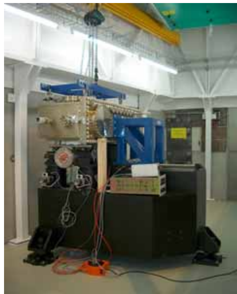
Fig. 8.3: Installation of microXAS mirror tank.
